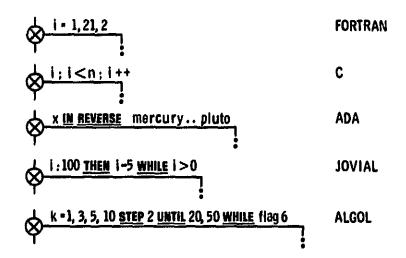
The last two examples illustrate hybrid loop-specifications. In fact, the Algol example uses all four loop forms! A basic Ada loop which requires some loop-body construct for termination might be represented as:
