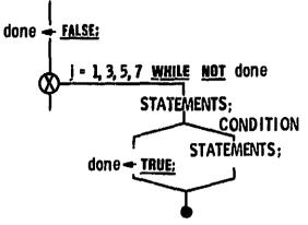
Some languages, e.g. Ada and HAL/S, permit a labeled escape which causes the **exit** of a nest of constructs to a forward point. HAL/S generalizes this to allow an **exit** from any labeled code block bracketed by **do and end**, thereby producing a forward **go to** by another name.
