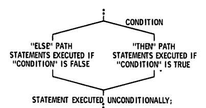
The "**else** path" may be null, in which case a line is drawn vertically joining the top and bottom portions of the symbol.
