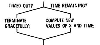
This example also illustrates the conditional form to be followed in a high-level D-Chart. That is, the condition should be posed as a question followed by a question mark. Also, while a code-level D-Chart should follow the syntactic forms imposed by a particular language, a high-level D-Chart may use more meaningful conditional and logical symbology, e.g. ">" instead of ".GT.".
