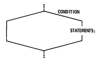
Either, or both, of the **then** (true) or **else** (false) paths may be any control structure which obeys the general structured rule of "one input path, one output path." Each **if-then-else** symbol should have an explicit join which causes the input and output paths to be aligned on the page. This join is made explicit in Fortran and Ada by **end if**, and replaces those keywords. Note also that this symbology removes any ambiguity arising from a "dangling **else**."
