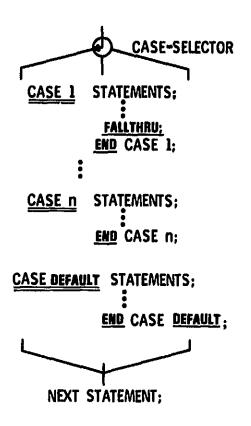
If the number of cases is very large, and/or the logic in the paths is extensive, it may be necessary to consider each case path as an "internal procedure" which stands alone following the entire D-Chart. This is particularly true if the **case** construct is embedded in a complicated logical nest. Each **case** symbol should be clearly commented and cross-referenced to its set of "internal procedures."
