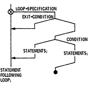
In a proper D-Chart an unlabeled escape may lead only to the statement following the loop in which it is contained, thereby satisfying the "one in, one out" rule. The escape construct can be avoided at the cost of a spurious boolean variable and two assignment statements in languages which permit hybrid loop-specifications. In this case, the escape path is directed to the loop end as follows:
