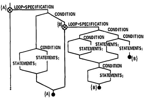
The conditional loop class requires further discussion. In the case of a loop-specification consisting only of a **while** condition, it is necessary to state only the logical expression, preceded optionally by the keyword **while**.
