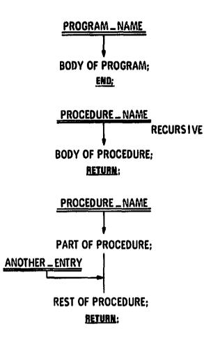
In appearance the most significant difference between a D-Chart and an ANSI Standard flowchart is the elimination of closed shapes, e.g. rectangles, diamonds, and circles. Sequential statements are written in free-form, one below the other as follows:
