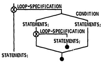
When the D-Chart involves nested loops in close proximity, some form of labeling should be supplied to clearly relate the switch-dot pairs. If the loop is labeled in the coding, the labeling convention previously discussed should be used. Otherwise, the labeling should be done by comments, where the "comment" need not be more than a single letter or number. Also as a matter of style, the dot should be placed as near to its switch as possible.
