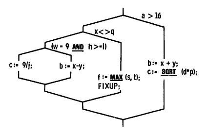
This example also illustrates that it may be desirable to enclose the "condition" in parentheses in order to avoid confusion between a statement to be executed and a condition to be tested, should statements and conditions be in close proximity.
