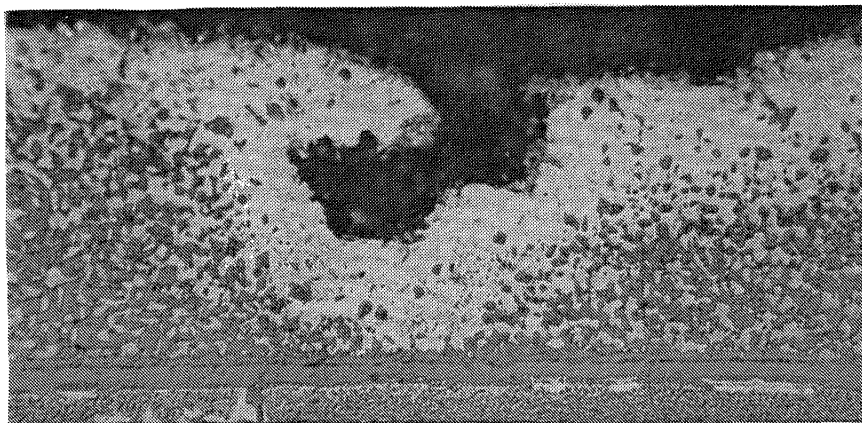
Figure 3. Photomicrographs of NiCoCrAlY coated specimens from hot corrosion burner rig test at 900° C showing progressive degradation with time.
