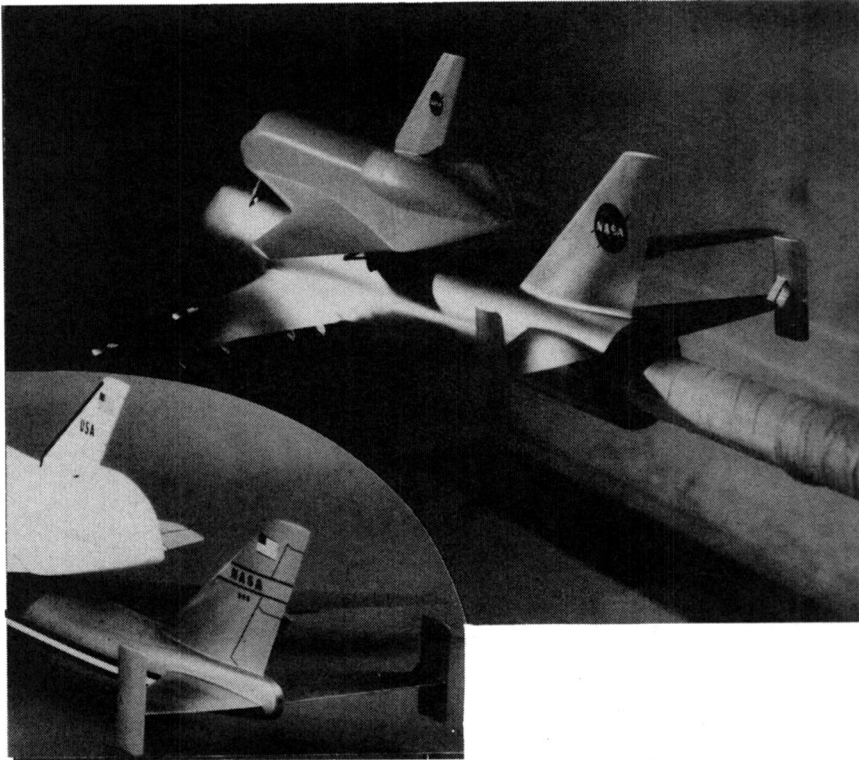
AFTERBODY ALTERATION OF THE COMBINED 747/SHUTTLE CONFIGURATION TO ACCOMMODATE A STING COMPATIBLE WITH THE HIGH COMBINED LONGITUDINAL AND LATERAL LOADS
