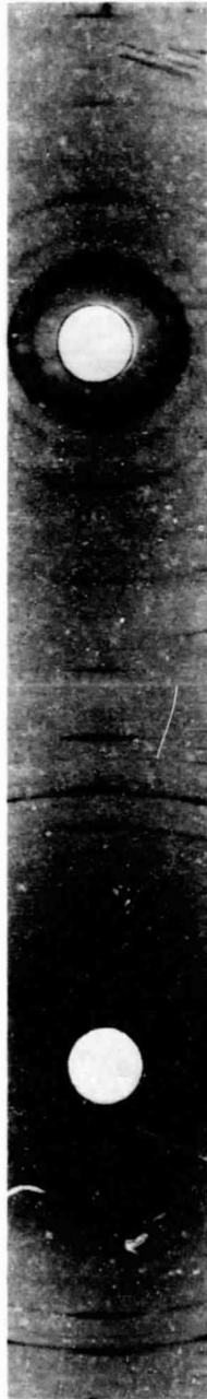
Fig. 29A X-Ray Powder Pattern of Isolated M_7C_3 Carbide Fiber, see Table 27
