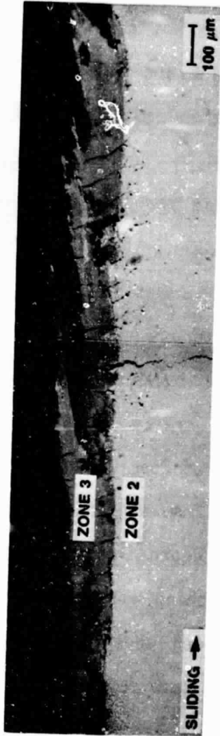
Fig. 43A Light Micrograph, Taper Section as Shown in Fig. 35B, N = 10,000 Cycles, D.S. at 25 \text{ cmh}^{-1}
