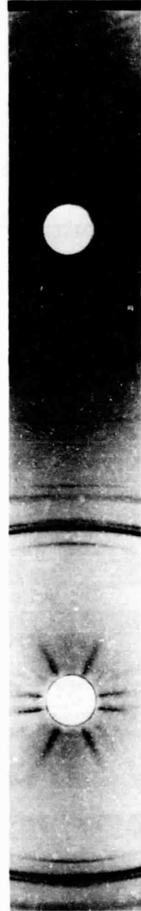
Fig. 29B X-Ray Powder Pattern of M_7C_3 in Matrix Needle, see Table 27
