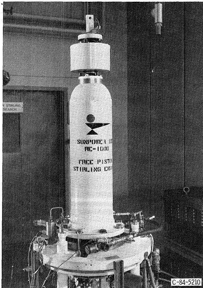
Figure 16. - Balance unit installed on NASA/Lewis Re-1000.
