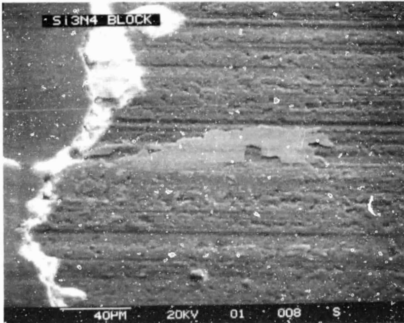
Fig. 3.2—Scanning electron microscope views of Si 3 N 4 wear track - run #31- 1200°F - 5000 rpm - upper - 50X; lower - 500X
