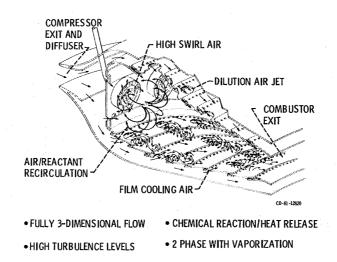
Figure 1. - Cutaway Illustration of a portion of a full annular combustor system, with major features highlighted.
