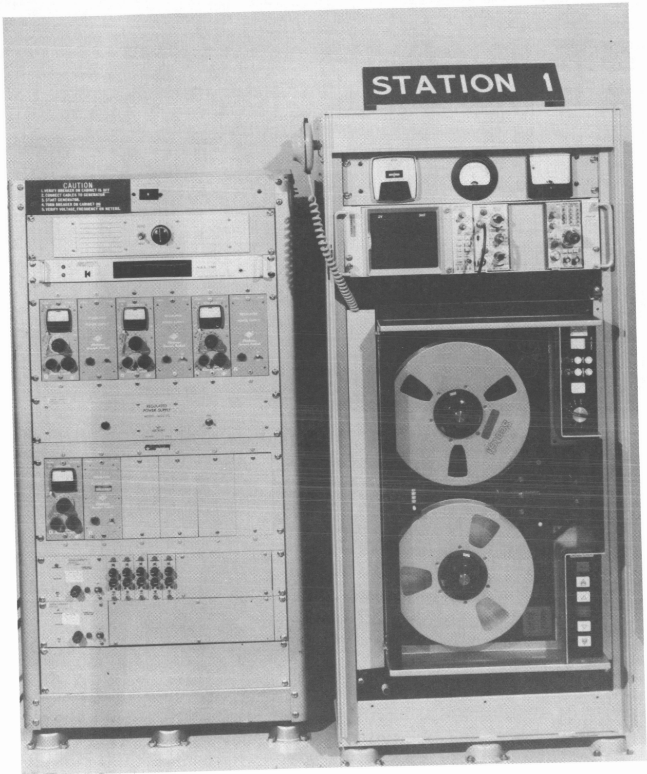
Figure 5.- Typical sonic boom data recording equipment.
