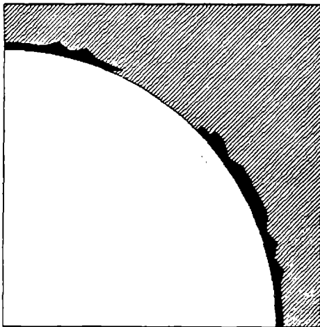
c) 25% interface degradation, yielding at 3.5 MPa
