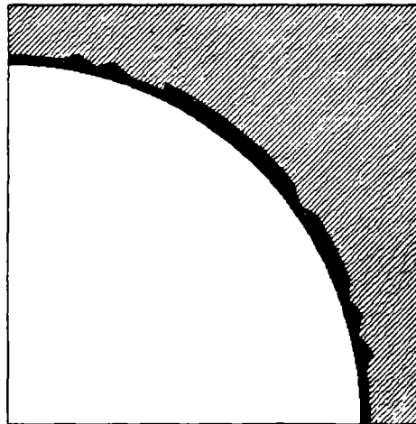
d) 25% interface degradation, yielding at 14 MPa
