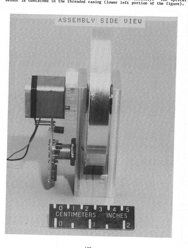
This photograph shows a side view of the wheel assembly. The optical sensor is contained in the threaded casing (lower left portion of the figure).
