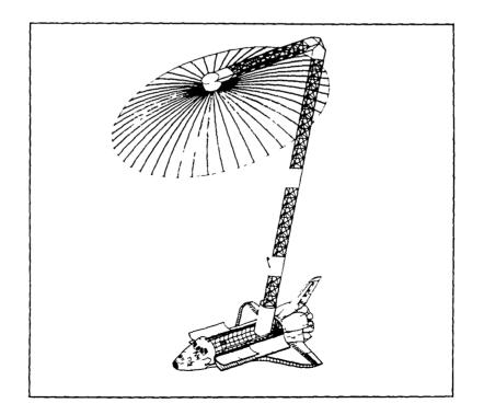
Fig. 2. Feed-attached flight experiment configuration.
