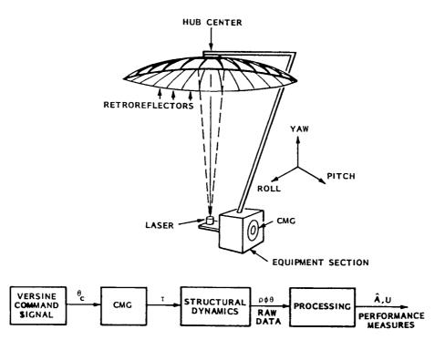
Fig. 16 Functional block diagram of slew experiment
