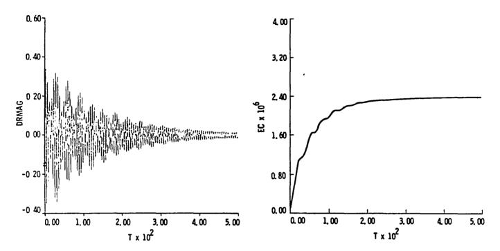
Figure 14. Variations of the Feed-Dish Distance and the Control Energy (EM Controller).
