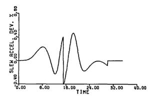
Fig. 9(a). Roll-axis Slew Acceleration Deviation during Roll-Axis BB Slew.  $t_1 = 15.038 = t_2$ ,  $t_3 = 30.075$ .
