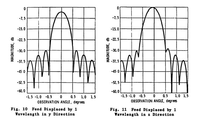
As can be noticed, displacements along the x and y axes produce significant variations in the gain while displacements along the z axis have almost negligible effects. It can thus be observed that, to optimize the gain most of the effort should be concentrated on controlling the feed displacements along the x and y directions and that the control along the z direction can be relatively loose.
