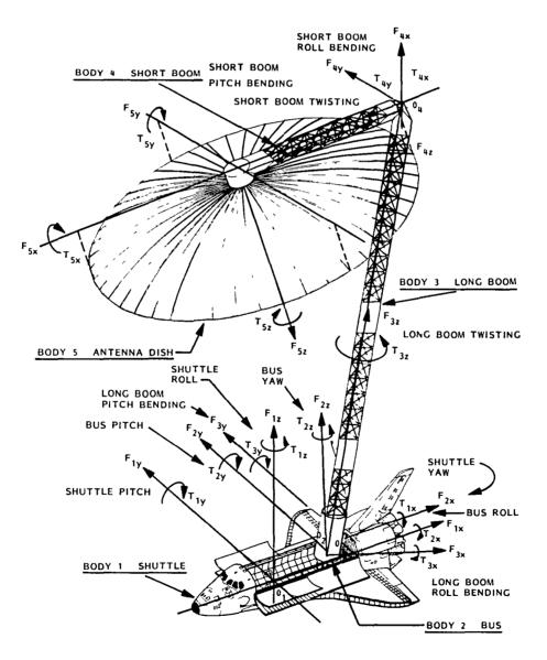
Fig. 11 A five-body system for the flight experiment
