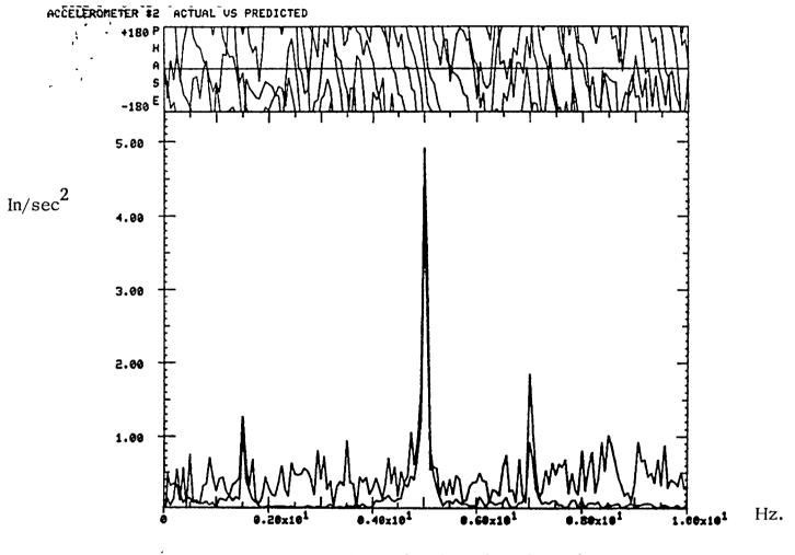
Fig. 9 Transform of actual and predicted accelerometer outputs
