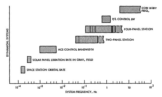
Fig. 9 Frequency characteristics of space station dynamical systems
