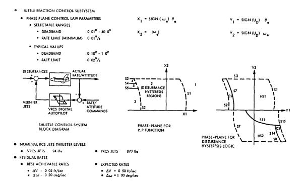
Fig. 10 Shuttle Reaction Control Subsystem and residual rates
