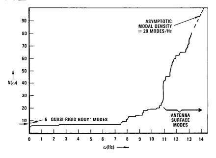
Figure 3. 15-M Model Cround Test Configuration Mode - Count Versus Frequency
