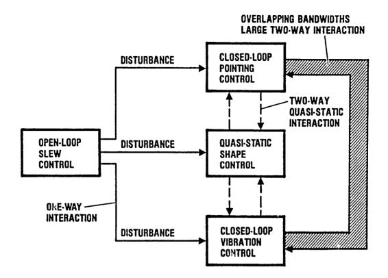
Figure 3. Control Subsystem Interaction for LSS
