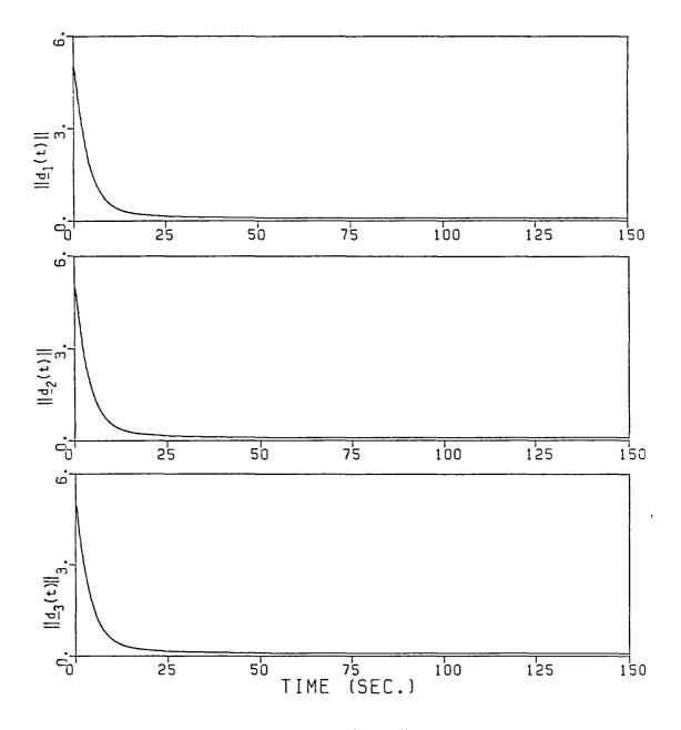
Fig.9a Time-domain behavior of  $||\underline{d}_{J}(t)||$ , j=1,2,3 for the final approach phase of modules 1 and 2 with feedback gains  $k_{\rho 0} = 2.2 \times 10^{6}$ ,  $k_{\rho 1} = 4$ , and  $\underline{d}^{d} = (0.1,0,0)^{T}$ .
