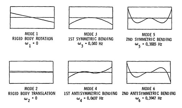
Fig. 8 Modal properties for the two-panel configuration model
