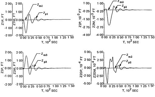
PLANT OUTPUTS CONVERGE TO THE ZERO STATE WELL WITHIN 100 SECONDS IN THE PRESENCE OF TRUNCATION, PARAMETER ERRORS, AND INSTANTANEOUS CHANGE OF MASS AND INERTIA BY MORE THAN 100%
