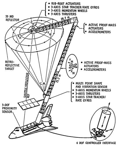
Fig. 21 Flight experiment architecture with 6-DOF controlled attachment interface 378
