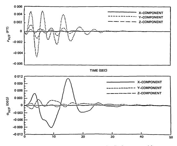
Fig. 14 Hub-to-feed linear and angular displacements with hub and feed controller configuration 2 365
