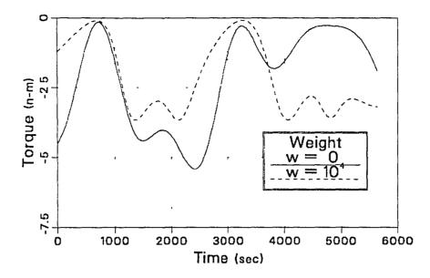
Figure 5. Magnetic Torquer Desaturation Torques in Pitch for w = 0and w = 10000
