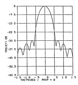
Fig. 16 Undistorted Antenna Pattern
