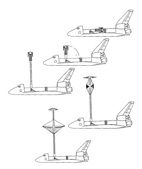
Figure 14. Flight Experiment Deployment Sequence
