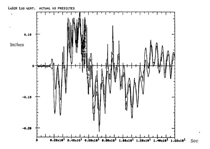
Fig. 6 Actual vs. Predicted Laser Line-of-Sight
