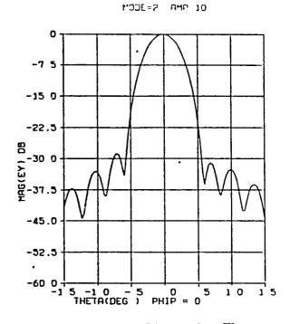
Fig. 19 Pattern Distortion When Mode 2 Amplitude = 10
