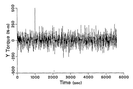
Figure 6. Crew, Docking, Aerodynamic and Gravity Gradient Disturbing Torques about the Pitch Axis
