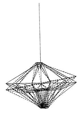
Figure 4. Mode 4: Cuasi-Rigid Rotation (f = 0.163 Hz)
