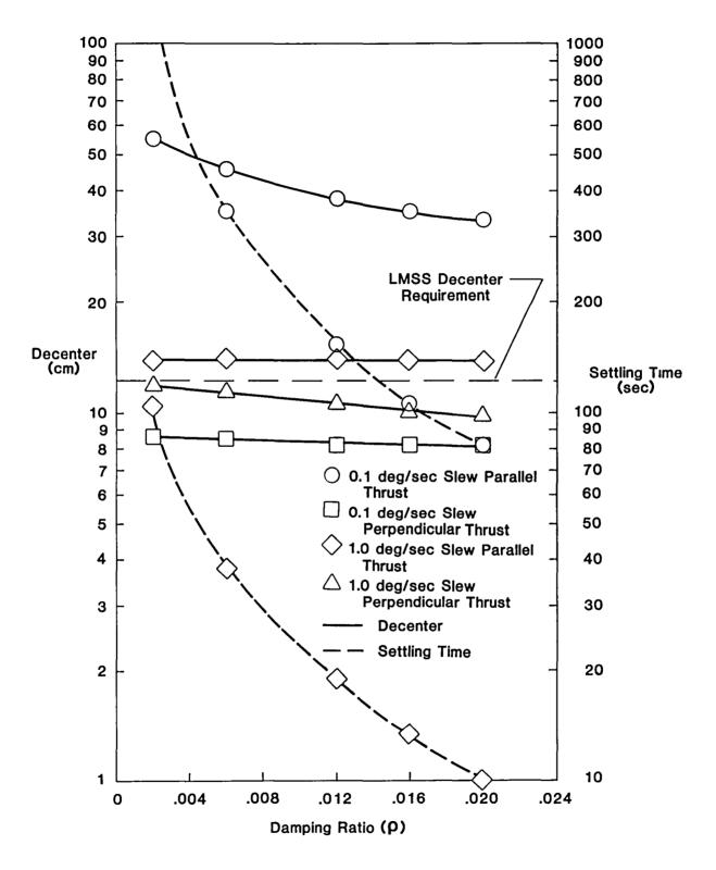
Figure 17. Damping Effects on Tetrahedral Truss Dynamic Response
