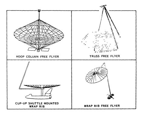
Fig. 1 Potential large space antenna flight experiment configurations.
