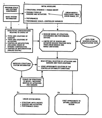
Figure 10. Initial Design Methodology: Closed-Loop Modeling and Sensor/Actuator/Control Logic Selection
