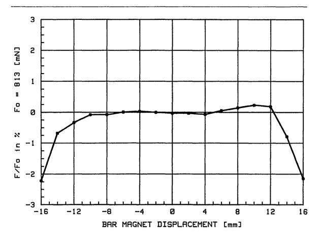
Figure 5. Magnetic force vs. displacement. Measurement results of dual coil system.
