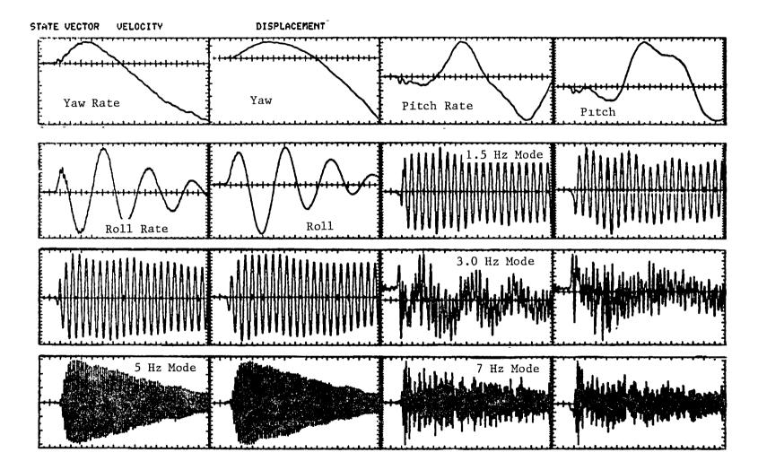
Fig. 5 Estimated State Vector-(Timespan is 16 sec, chirp applied at t=2 sec)
