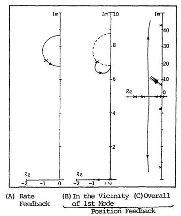
Fig. 7 Results of Damping Ratio Measurements Compared with Numerical Results for Direct Rate and Position Feedback.
