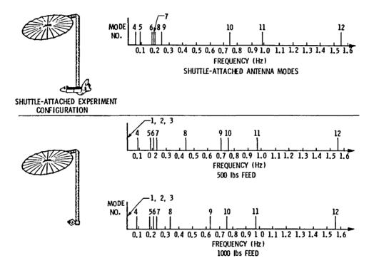
Fig. 19 Modal frequencies of a shuttle-attached system and two free flier antennas
