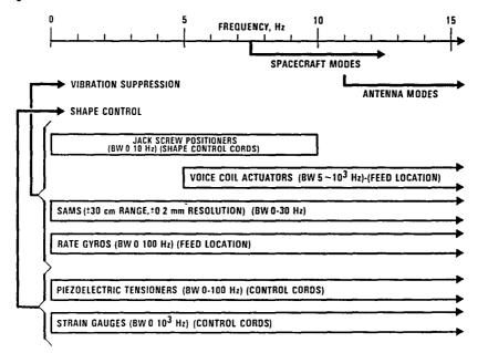
Figure 9. Selection of Actuators and Sensors For Vibration Suppression and Shape Control (With Bandwidths).
