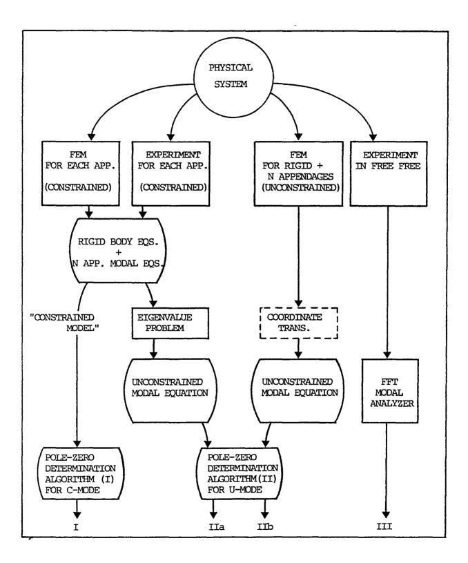
Fig. 1 Approaches for Modeling and Pole/Zero Determination
