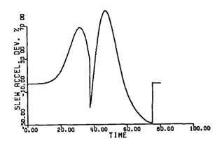
Fig. 9(c). Yaw-axis Slew Acceleration Deviation during Yaw-Axis BB Slew.  $t_1 = 37.688 = t_2$ ,  $t_3 = 75.376$ .
