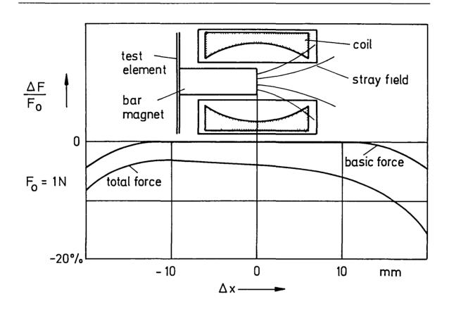
Figure 3. Magnetic force vs. displacement. Numerical results, single coil.
