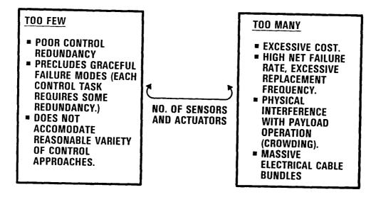
Figure 8. Number of Sensors and Actuators (Some Guidelines)
