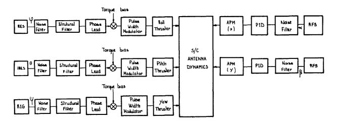
Figure 5 : 1<sup>st</sup> CONTROL CONCEPT: SEPARATE BODY ATTITUDE AND ANTENNA BEAM CONTROL LOOPS
