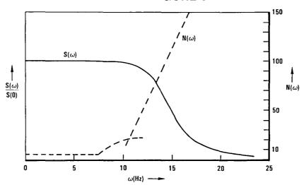
Figure 7. Suggested Broad-Band Disturbance Spectrum for 15-M Ground Test (Applied Independently Along X and Y axes)
