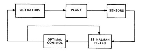
Fig. 10 LQG control system block diagram
