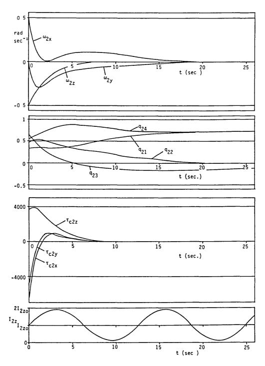
Fig.6 Time-domain trajectories of module 2 with attitude control law (74),initial conditions and feedback gains given in Fig.7, and with perturbed I<sub>2z</sub>(t)=1.68772×10<sup>4</sup>(1+0.95 sin(t/2)) (kg.m<sup>2</sup>)
