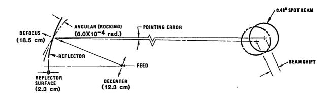
Figure 9. Antenna Accuracy Requirements
