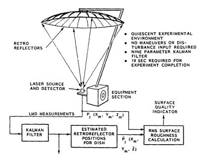
Fig. 4. Functional diagram of geometry identification experiment.
