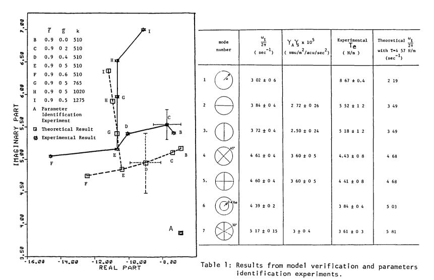
Figure 5: Comparison between experimental and theoretical pole locations.
