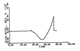
Fig. 10(b). Pitch-axis Slew Acceleration Deviation during Pitch-Axis BB Slew (Experiment b).
