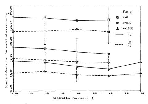
Figure 6: Comparison between theoretical and experimental standard deviation for modal observation y<sub>2</sub>.
