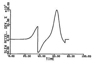
Fig. 9(b). Pitch-axis Slew Acceleration Deviation during Pitch-Axis BB Slew.  $t_1 = 37.435 = t_2$ ,  $t_3 = 74.871$ .
