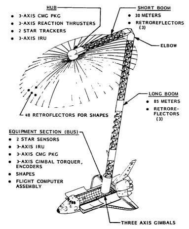
Fig. 17 Flight experiment hardware configuration
