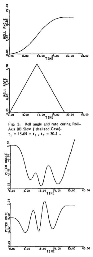
Fig. 4(b). Induced pitch angle and rate during Roll-Axis BB Slew.
