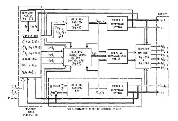
Fig.4 Block diagram of the proposed automatic terminal rendezvous control system.
