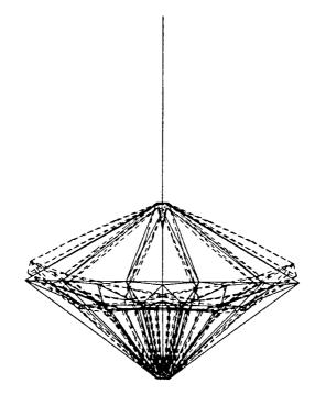
Figure 5. Mode 6: First Hoop Bending (f = 7.493 Hz)
