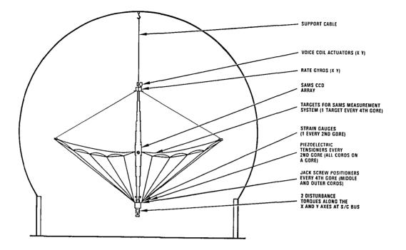
Figure 2. 15-Meter H/C Model Cable Suspended Configuration for Ground Testing
