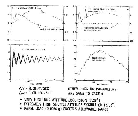
Fig. 14 Dynamic responses of soft docking with expected approaching rates (Case 8)
