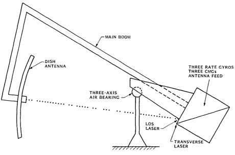
FIG. 2 Schematic of POC Test Specimen
