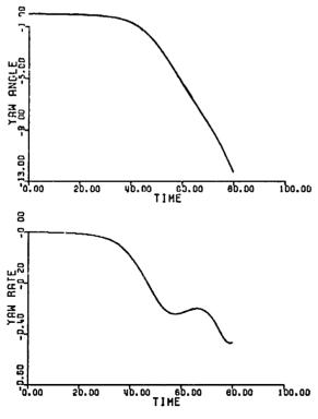
Fig. 11(c). Induced yaw angle and rate during Pitch-Axis BB Slew (Experiment b).
