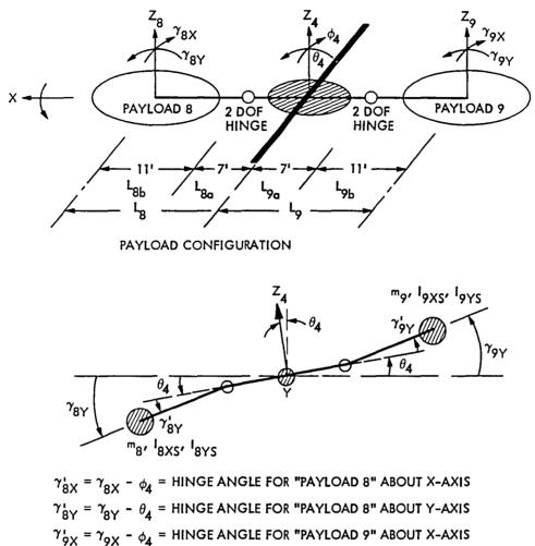
$\gamma'_{9Y} = \gamma_{9Y} - \theta_{4}$  = HINGE ANGLE FOR "PAYLOAD 9" ABOUT Y-AXIS
