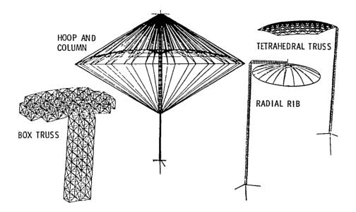
Figure 1. Antenna Structural Concepts
