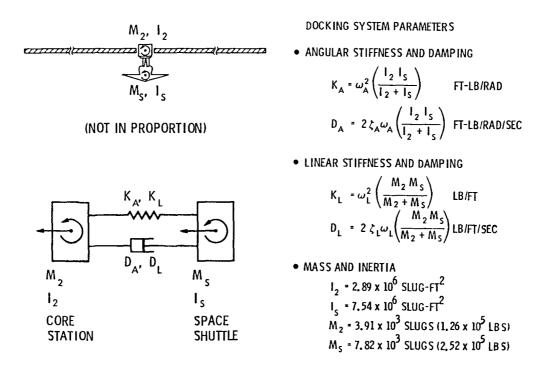
Fig. 12 Soft docking design and system parameters
