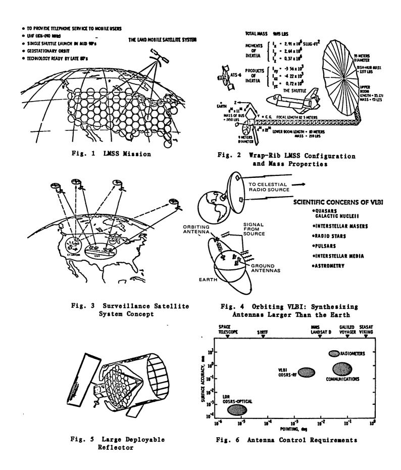
is slightly more stringent, and the pointing accuracy tighter by an order of magnitude. For LDR, the pointing accuracy is about  $10^{-5}$  degree (0.04 arc second), similar to the one required for the Space Telescope. The RMS surface error, however, is in the sub-micron region.
