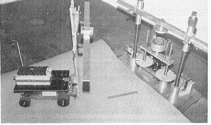
Figure 5. Radio-Controlled Forklift, carrying test specimen to launching device(note six-inch ruler in foreground)
