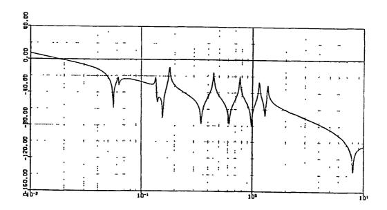
Figure 6 : CENTRAL BODY TRANSFER FUNCTION USING P.D NETWORK AND CAUER FILTERING (1<sup>st</sup> control concept)
