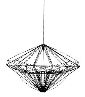
Figure 6. Mode 10: Higher-Order Hoop Bending (f = 8.029 Hz)
