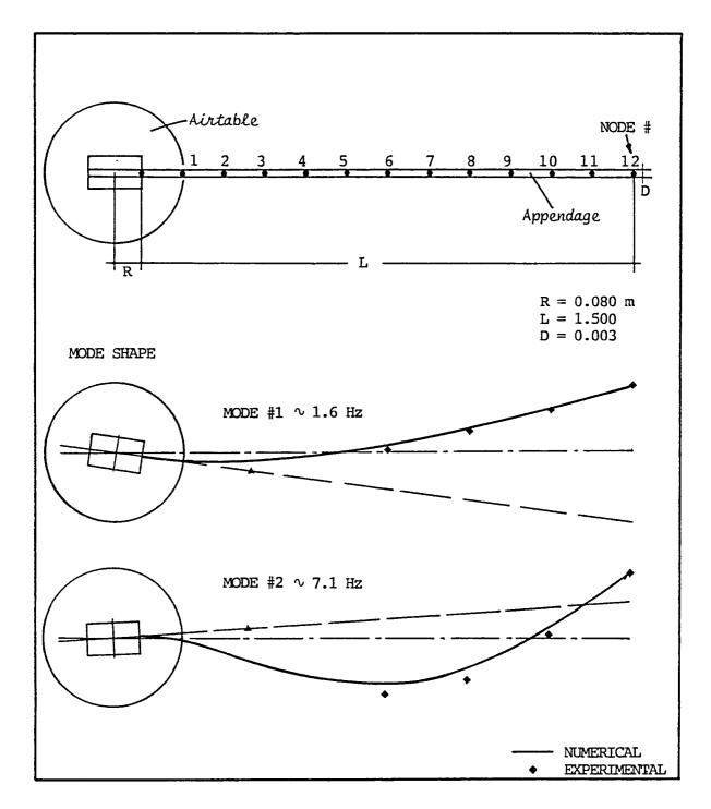
Fig. 3 Appendage Dimension and Unconstrained Vibration Modes
