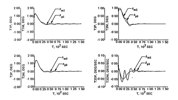
(b) Plant and model rotational state responses Fig. 16 Adaptive regulator control simulation with initial transient
