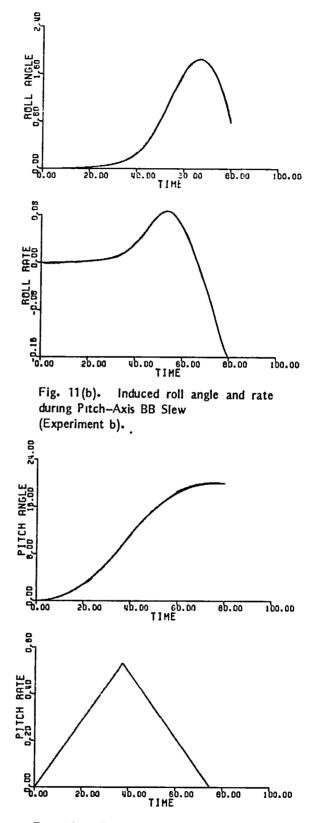
Fig. 12. Pitch angle and rate during Pitch-Axis BB Slew (Experiment c).
