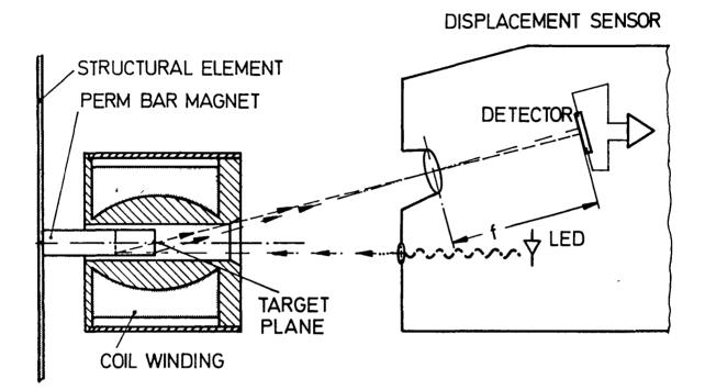
Figure 4. Principle of displacement measurement.
