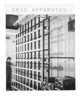
To date, experiments have been conducted to define the dynamics of the grid. An air jet was used to excite the grid at several frequencies impinging on it at point 1, normal to the plane of the grid. For each frequency, the excitation was applied until a 1 inch amplitude was obtained. Then, the excitation was removed and records were made of the output of 9 noncontacting position sensors located at points 1 through 9.
