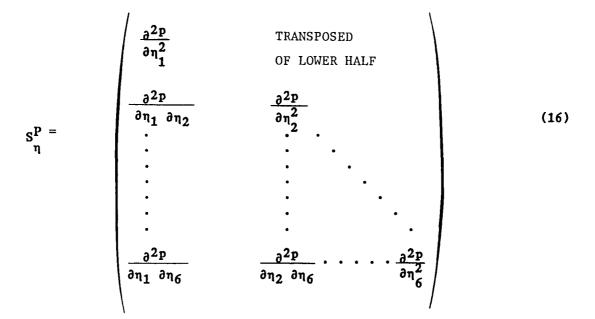
Each element of the sensitivity matrix is computed by tabulating the values of the peak electric field as a function of the corresponding modal amplitudes about  $\eta_1 = \eta_2 = \dots = \eta_6 = 0$  and then using the bi-cubic spline function to interpolate P. The second derivatives are then obtained from the spline coefficients.
