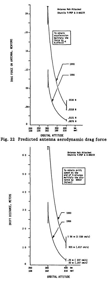
Fig. 23 Predicted 5-minute shuttle-antenna separation distance due to aerodynamic effect
