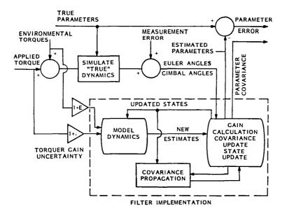
Fig. 6. Performance evaluation block diagram for mass properties identification.
