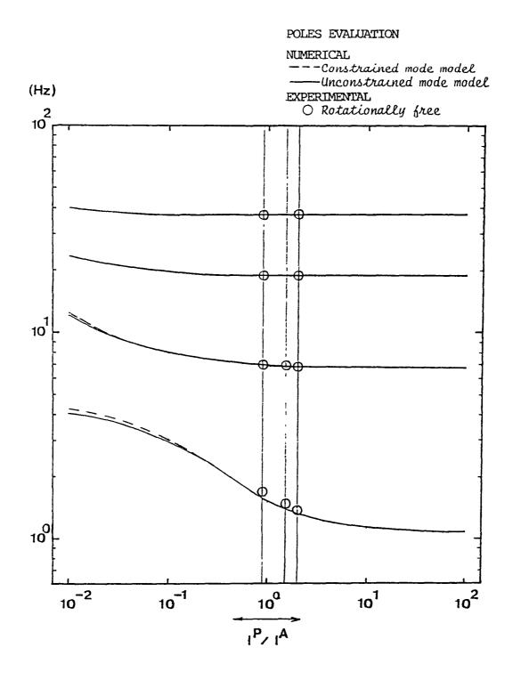
Fig. 4 Comparison of the Poles Determination by the 4 Modes
