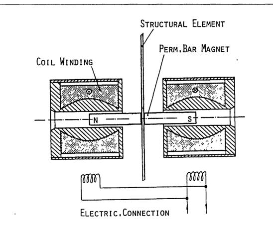
Figure 2. Electrodynamic force actuating system.
