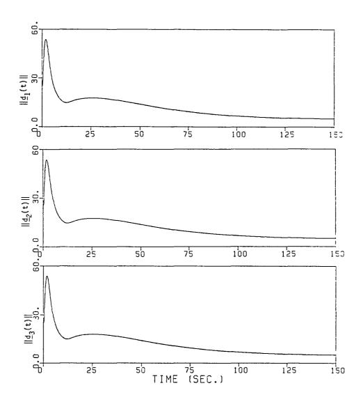
Fig.8a Time-domain behavior of  $\|\underline{d}_{j}(t)\|$ , j=1,2,3 corresponding to motions of modules 1 and 2 shown in Figures 7 and 5, and initial conditions for relative translation given by  $[\underline{\rho}(0)]_{1} = (50,0,5)^{T} \text{m.}, [\underline{\dot{\rho}}(0)]_{1} = (0,-5,0)^{T} \text{m./sec.,and}$ feedback gains:  $k_{\rho 0} = 2.2 \times 10^{6} \text{ and } k_{\rho 1} = 40.$
