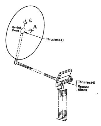
Figure 6: OMSAT Actuator Configuration
