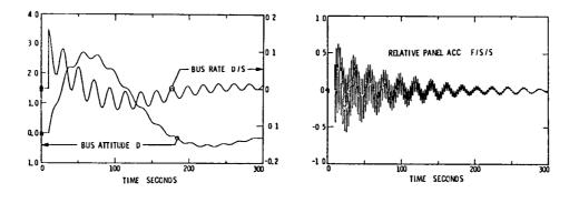
$\Delta V = 0.05 \text{ FT / SEC}$  $\Delta \omega = 0.20 \text{ DEG / SEC}$  SHUTTLE COASTING BEFORE CONTACT STATION CONTROL BW = 0.005 Hz
