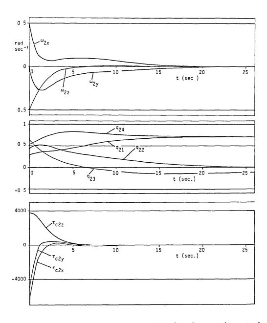
Fig.5 Time-domain trajectories of module 2 with attitude control law (74) and initial conditions:  $[\underline{\omega}_2(0)]_2 = (0.5, 0, -0.5)^T$ rad./sec.,  $[\underline{\omega}_2^d]_2 = \underline{0}$ ,  $\underline{q}_2(0) = (\sqrt{0.1}, \sqrt{0.2}, \sqrt{0.4}, \sqrt{0.3})^T$ ,  $\underline{q}_2^d = (1/\sqrt{2}, 0, 0, 1/\sqrt{2})^T$ ;
