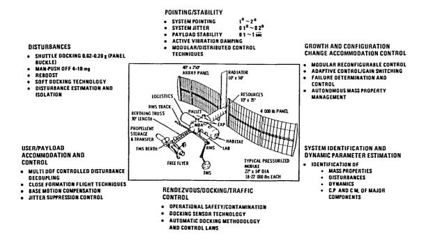
Fig. 1. Space station operational environment and control issues
