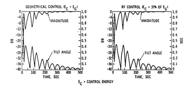
Figure 15. Comparison of the Tilt Angle and the Magnitude of the Electric Field.
