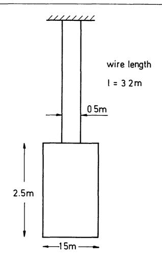
Figure 1. Vertically suspended plate.
