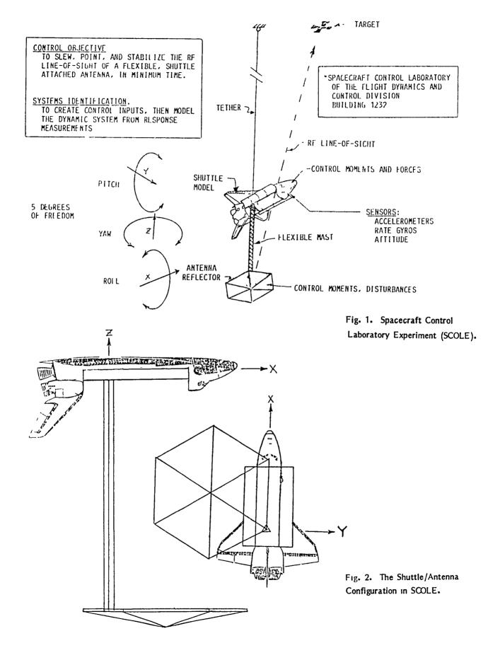
applied the standard theory of time-optimal control to each of the Shuttle body axes separately, but made an extension to encompass various bang-pause-bang control.
