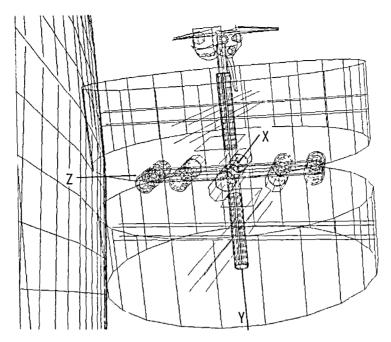
Figure 1. The Dual Spin Space Station with a Docked Orbiter
