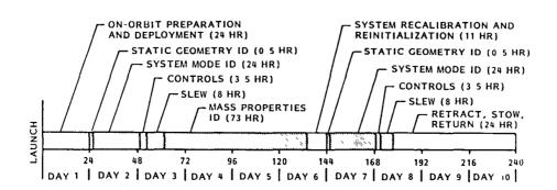
Fig. 18(b) "Nominal performance" flight experiment timeline with contingency times set to zero. Nine day flight plan
