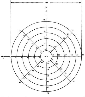
Fig. 3 Retroreflector targets layout on antenna reflector
