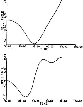
Fig. 8(b). Induced roll angle and rate during Yaw-Axis BB Slew.
