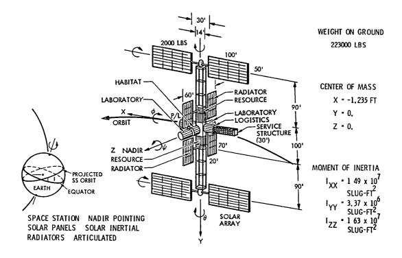
Fig. 2 Four-panel planar configuration
