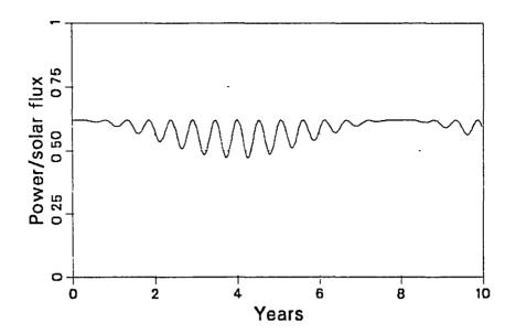
Figure 3. The Average Power Over One Orbit as a Function of Time
