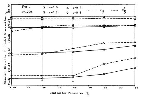
Figure 8: Comparison between experimental and theoretical standard deviation for modal observation y<sub>5</sub> at different synthesized spillover levels.
