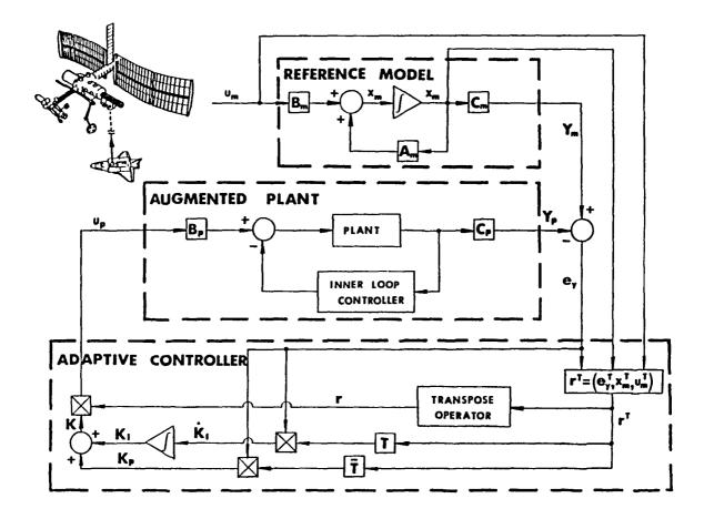
Fig. 15 Space station adaptive control system block diagram
