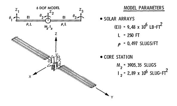
Fig. 7. Finite-element model for the two-panel configuration
