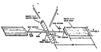
Figure 1. Control Configured Space Station
