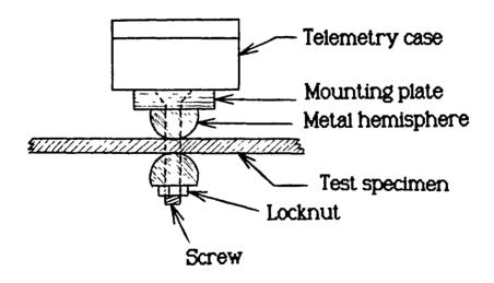
Figure 3. Telemetry Support Geometry
