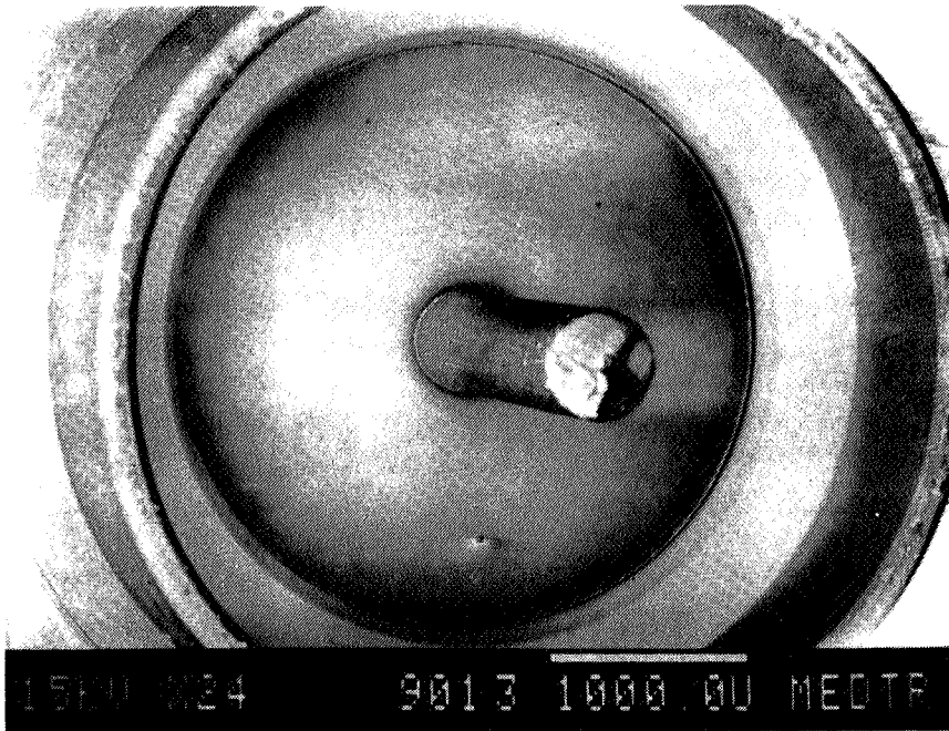
Figure 4. Glass Seal From Fresh Battery.
