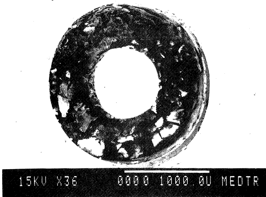
Figure 5. Glass Seal After Exposure to Liquid Electrolyte
