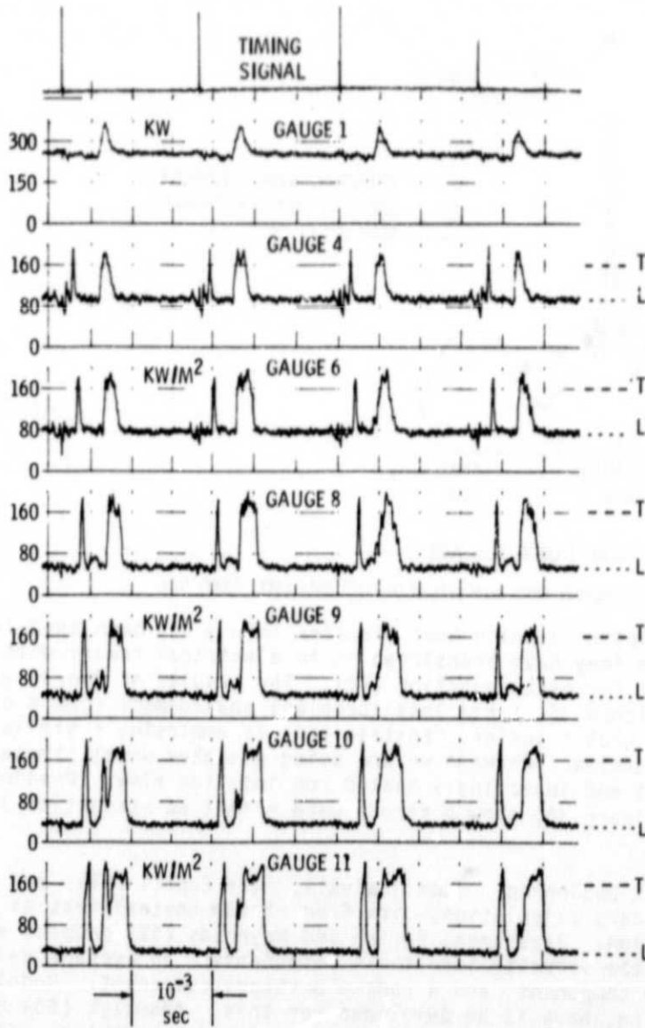
FIGURE 35. Unaveraged heat transfer traces with isolated wake and shockwave passing (two 0, 9 mm-dia-bars). (Ref. 48.)
