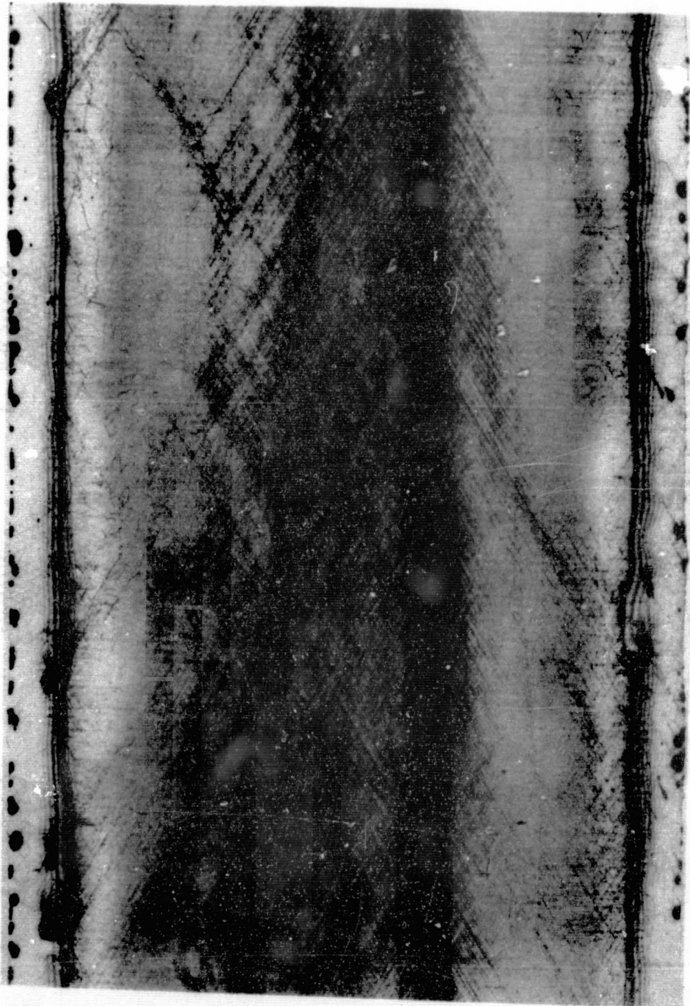
Fig 7b SOT X-ray topograph of medium quality web. Electrical data in Fig. 9.
