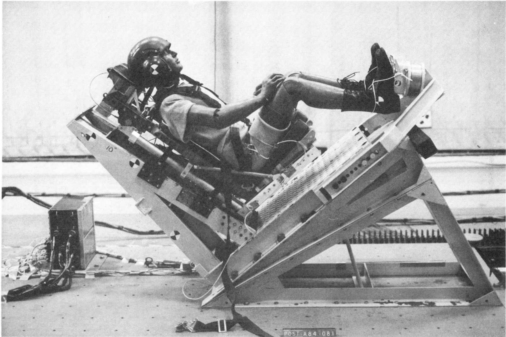
Figure 23. Energy-absorbing seat after CAMI test.
