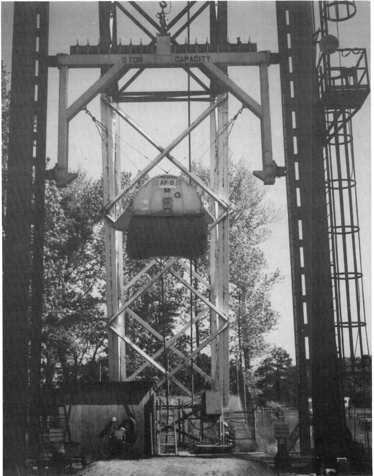
Figure 50. Drop tower of Impact Dynamics Research Facility at NASA Langley Research Center.
