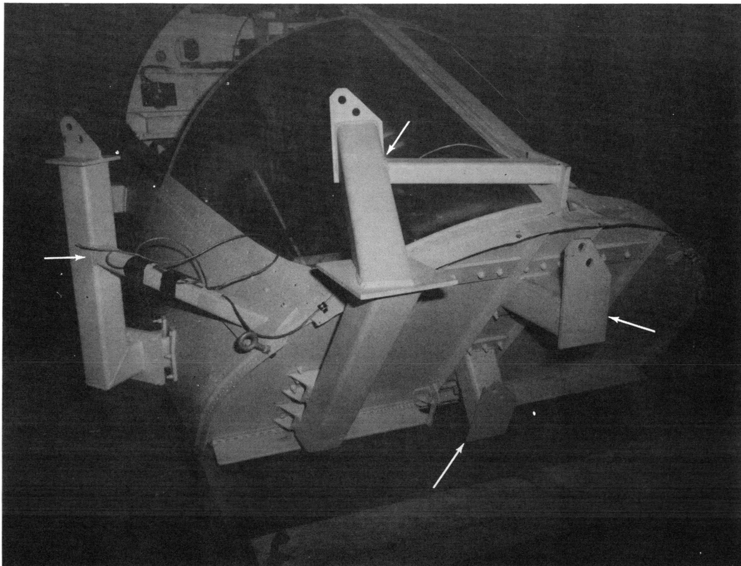
Figure 51. Structure at front of crew module added for attachment of attitude control cables.
