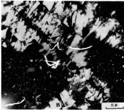
Figure 4. - Bright field TEM micrograph showing \gamma -Ni (fcc) grains in hypoeutectic alloy in the near wheel side region of the ribbon.
