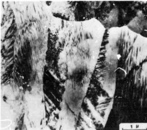
Figure 5. - Typical faulted \gamma -fcc Ni grains in hypoeutectic (near-wheel side), eutectic (near-wheel side) and hypereutectic (midsection) alloy ribbons.
