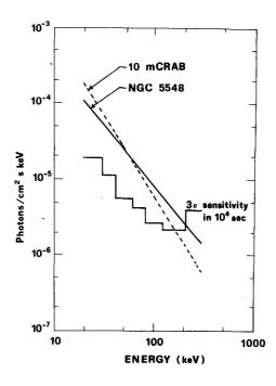
Fig. 1. - Spectrum determination sensitivity of the instrument with the rocking collimators
