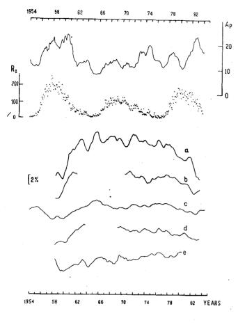
Geomagnetic activity (A\_-index), sunspot number R and the galactic cosmic ray intensity smoothed in annual interval on Yakutsk measurements by the muon telescopes (vertical) at 0, 7, 20 and 60 m w.e. depths (a,b,d,e, respectively) and by ionization chamber (c)
