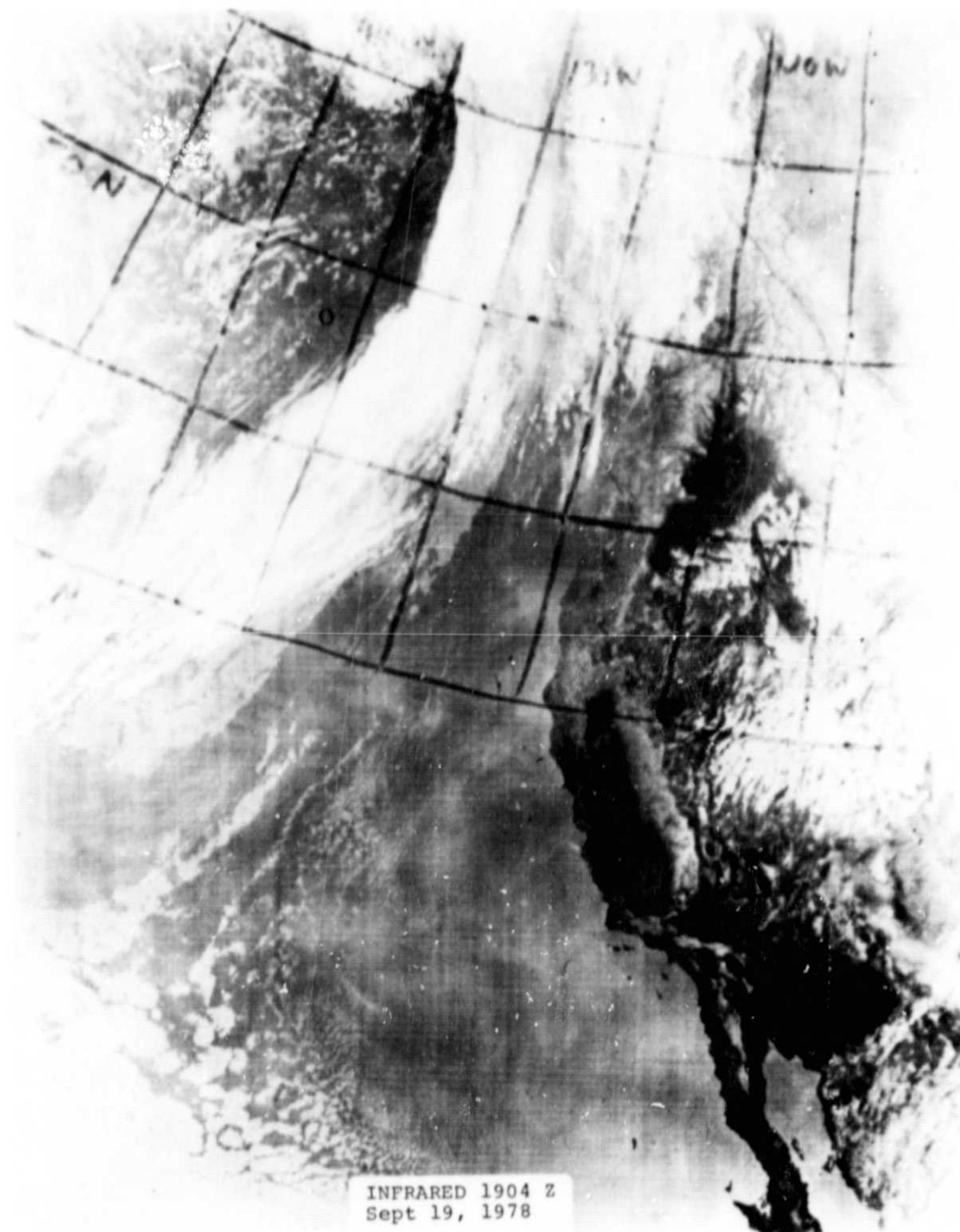
Figure E4-2. An Infrared Image of the Cloudy, Windy Sea - Near Land. (The black ellipse appearing in the upper left quadrant is the center of the swath (scan angle = 0^{\circ} ) as shown in dashed lines in Figure E4-1.)
