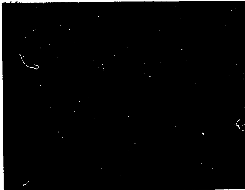
Figure 74. Pb X-ray Dot Map of the Carbon Fibers shown in Figure 73; 3200X.
