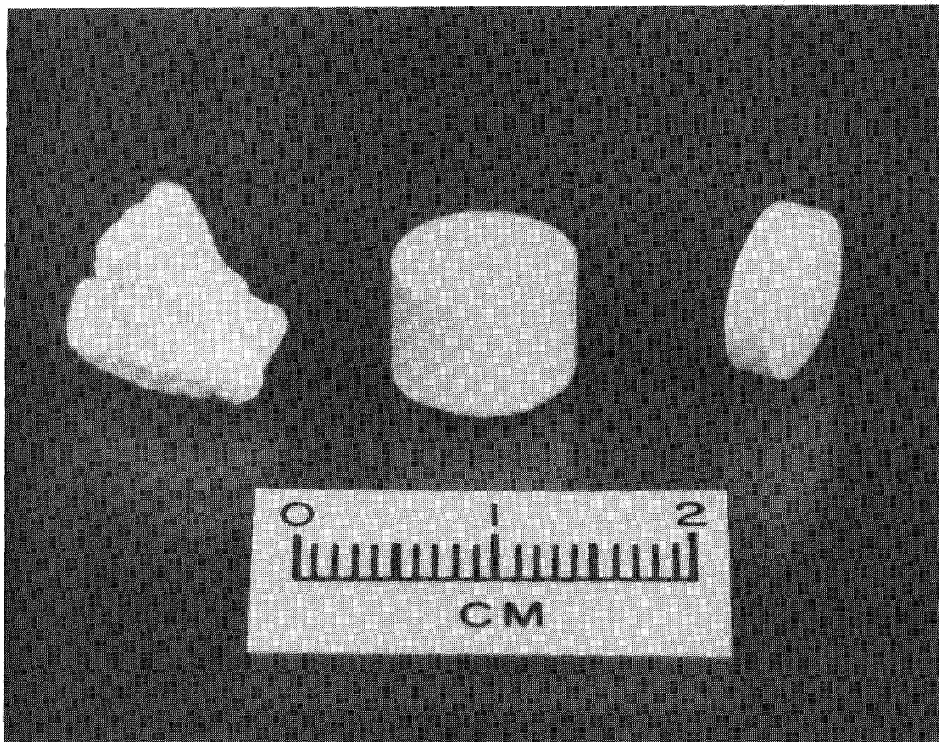
Figure 2.- Superoxide test-sample types: laboratory-fabricated pellet (center), commercial KO 2 granule (left), and tablet (right).
