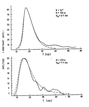
Fig. 2. shows a comparison of experiment and simulation for a shower with  $N_e = 6 \times 10^5$ ,  $E = 8 \times 10^{15}$  eV and S= 1.56. The N(x) profile has  $H_m = 7.4$  km and depth of maximum 470 gcm<sup>-2</sup>.
