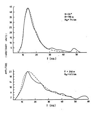
Fig. 3 shows a comparison and experiment and simulation for a shower with Ne =  $1.7 \times 10^6$ , E=  $3 \times 10^{16}$  eV and S= 1.19. The N(x) profile has HM = 7.4 km and depth of maximum 490 gcm<sup>-2</sup>.
