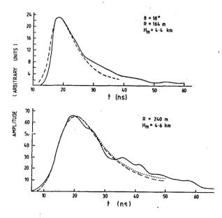
Fig. 1 shows a comparison of the experimental trace (full lines) for a shower with  $N_e = 4.6 \times 10^6$ ,  $E = 2 \times 10^{16}$  eV and S=1.28, and the Patterson-Hillas simulation using 10 GeV subshowers (dashed lines) and 100 GeV subshowers (dotted). The N(x) profile used<sup>1</sup> has  $H_m = 4.5$  km, and depth of maximum 640 gcm<sup>-2</sup>.
