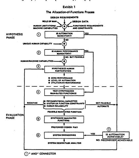
In the procedure, initial decisions identify these functions which must be allocated to man or machine for obvious reasons. Such allocations must be made to automation (Step 1) for instance, when regulation or policy requires it, when hostile environments preclude the presence of man, or
