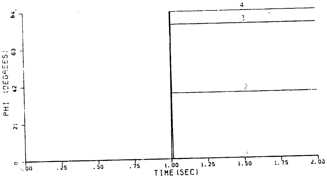
Figure 4-42: Detection Filter #5. No Unmodeled Modes. Actuator 1 Failure at T = 1 sec.. Output Filtering
