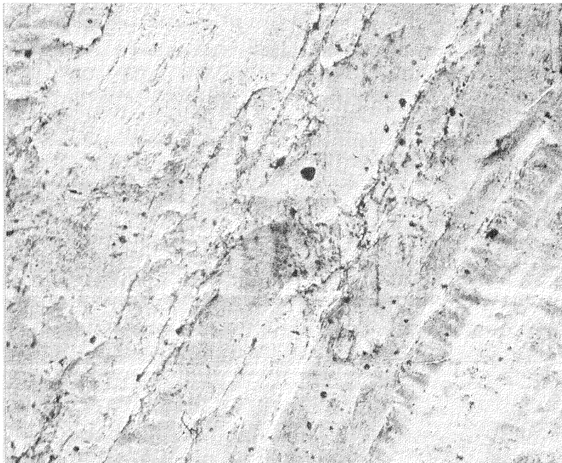
Figure 6. - Pt/Y 2 O 3 surface after 1000 hr at 1400 °C in H 2 (200X).
