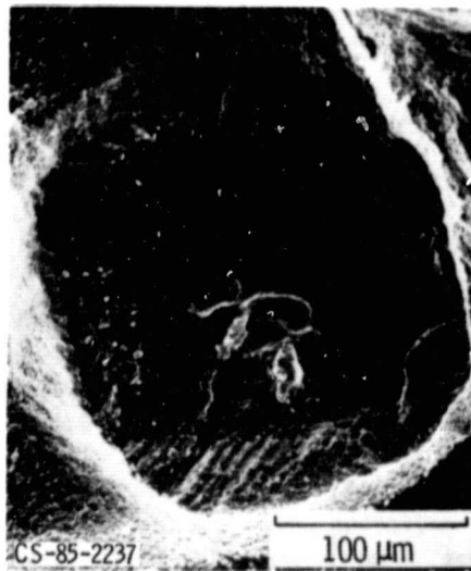
(b) SEM photomicrograph of a single crack initiation site.
