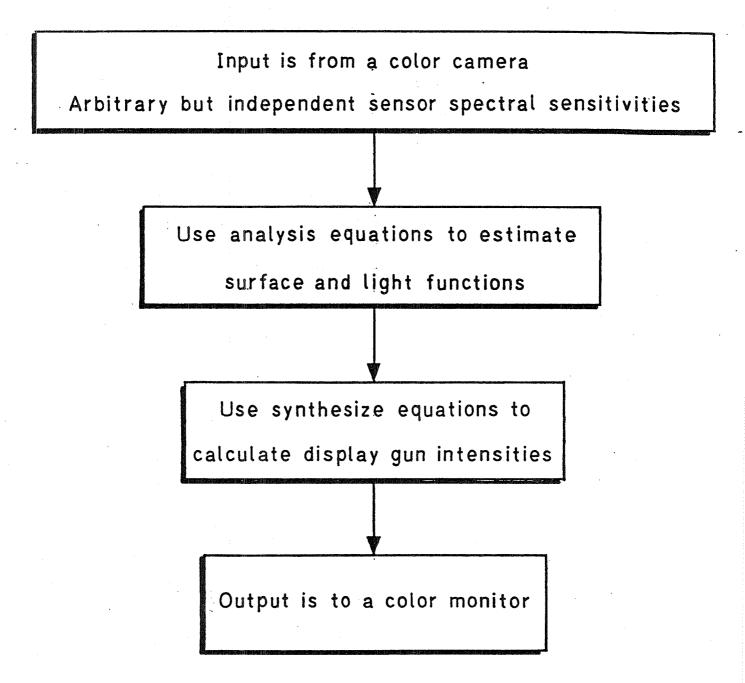
Figure 6. Flow diagram of how the analyses and synthesis procedures may be used together to convert the outputs of a camera with arbitrary sensor spectral to display an image so that it will appear to an observer as if he were at the camera position.
