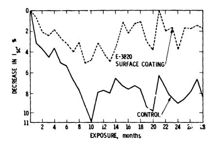
Outdoor Soiling Behavior of Tedlar 100BG30UT Piastic Film With & Without Fluorocarbon Antisoiling Coating
