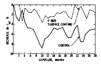
Outdoor Soiling Behavior of Glass With & Without Fluorocarbon Antisoiling Coating
