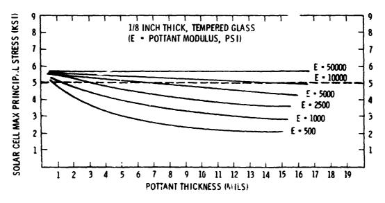
DOTTED LINE - ALLOWABLE CELL STRESS IN TENSION
