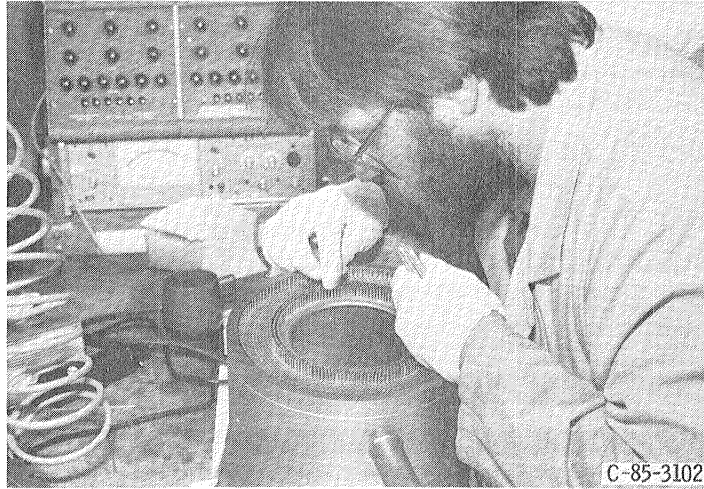
Figure 12. - Assembly of SPDE molten salt heat exchanger.
