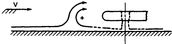
Fig. 11 Formation of ground vortex.
