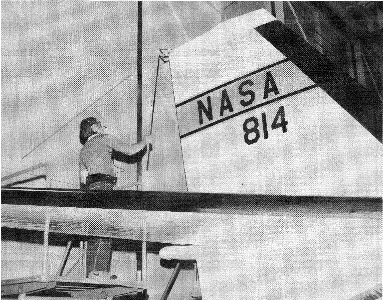
Figure 13. Roving wand being used to measure vertical tail motion.
