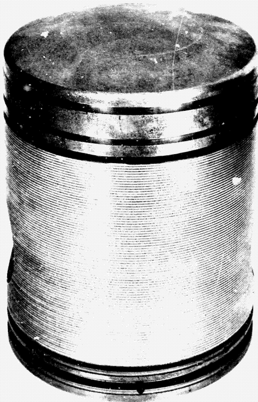
Figure 4.2-20. "BOKOR" Finish of Piston Skirt for Oil Retention
