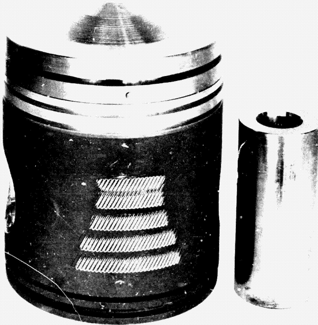
Figure 4.2-9. Piston Skirt with Knurling for Lubricant Retention
