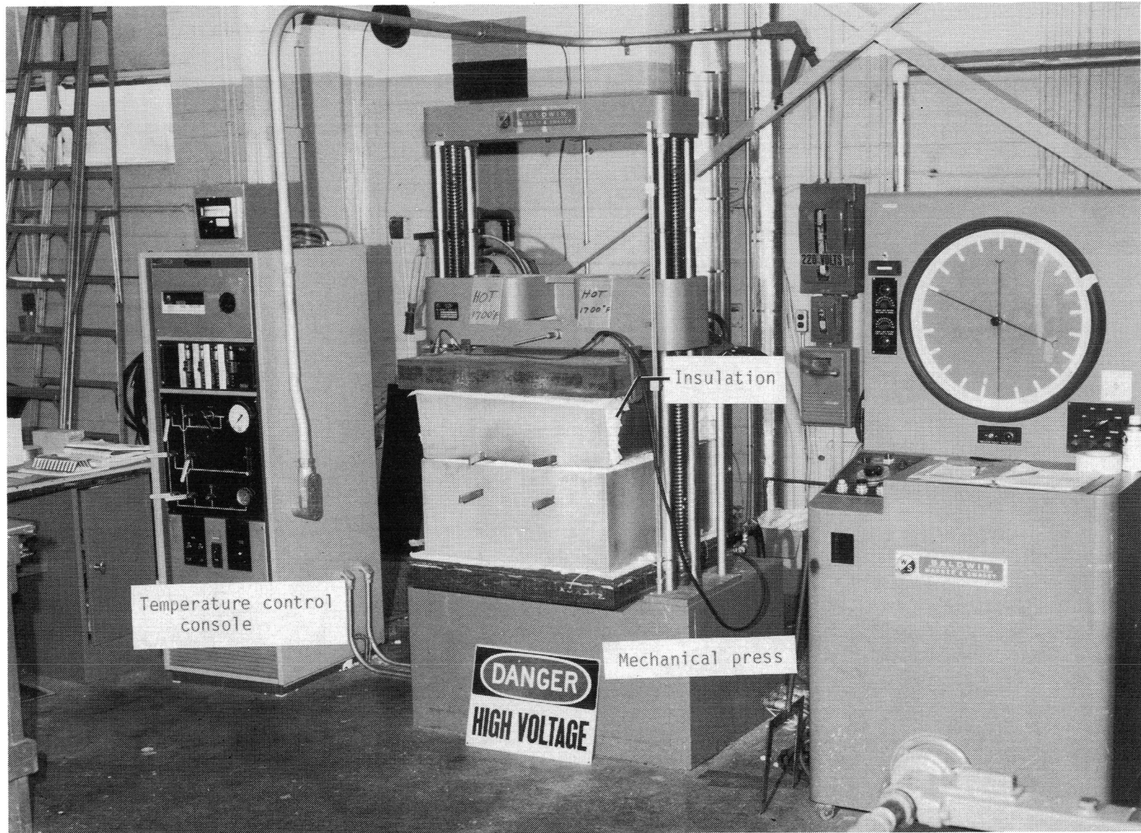
Figure 6.- Superplastic forming equipment to form half-hat elements.
