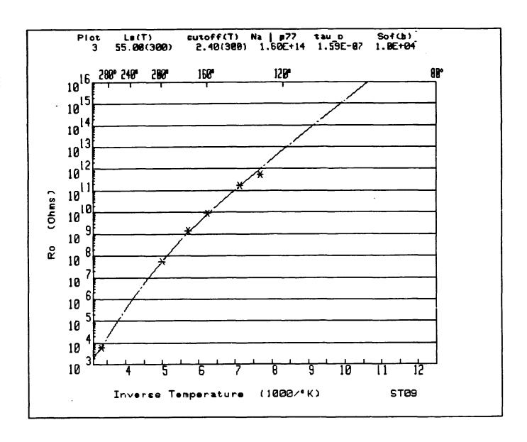
FIGURE 2. ANALYSIS OF THE Ro TEMPERATURE SHOWS LOW GENERATION RECOMBINATION CURRENTS ARE RESPONSIBLE FOR EXCELLENT MODERATE TEMPERATURE PERFORMANCE.
