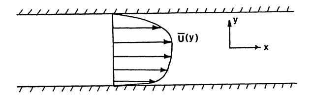
FIGURE 1. Fully-Developed Turbulent Channel Flow Subjected to a Spanwise Rotation after Johnston, Halleen, and Lezius (1972).
