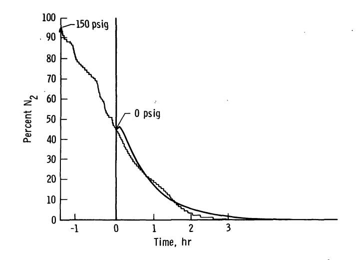
Figure 2(b). Percent N<sub>2</sub> in Evaporated Vapor Passing Through the N<sub>2</sub> Analyzer Versus Time: Test # 2. Wavy Line: Measured. Solid Line: Best Fit to Equation 9.
