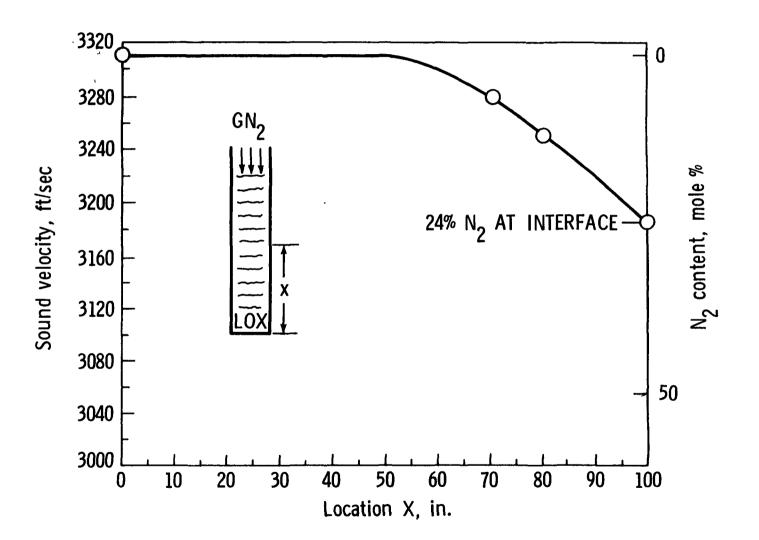
Figure 3. Contamination Profile Resulting From N<sub>2</sub> Pressurization of LOX at 1500 psi for 5 Min, in the 7-Inch Run Tank.
