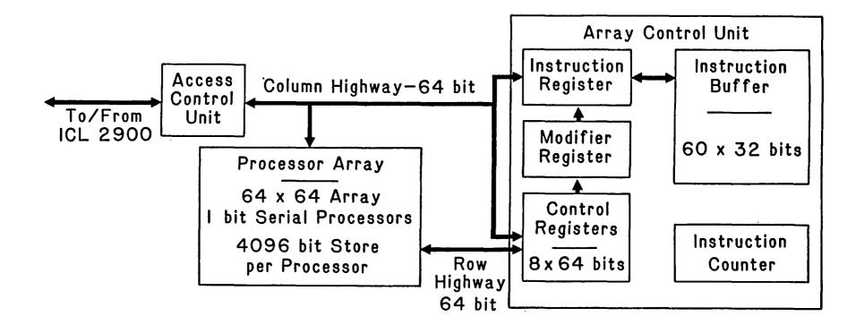
Figure 2. Schematic diagram of the DAP architecture.
