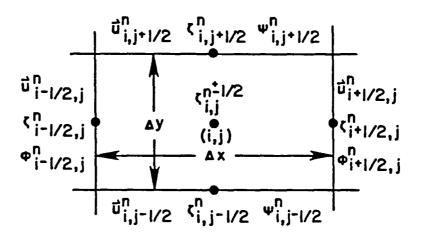
Figure 1. Typical computational cell and the data values associated with it.
