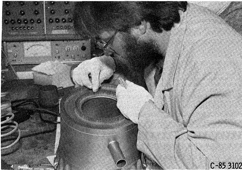
Figure 9. - Assembly of SPDE molten salt heat exchanger.
