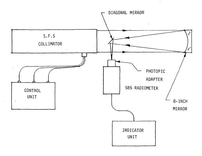
Figure 5. Collimator output calibration.
