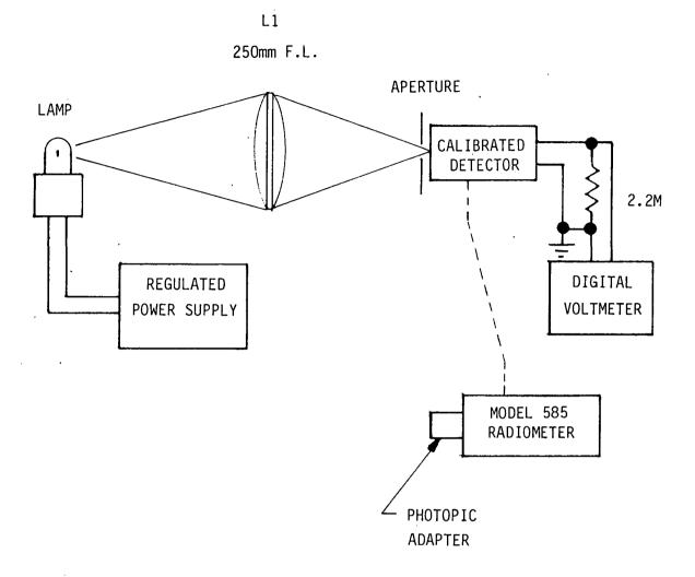
Figure 4. Photopic calibration of radiometer.
