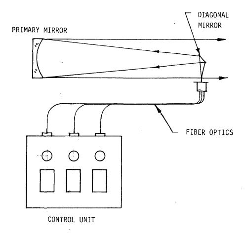
Figure 2. Schematic diagram of simulator.
