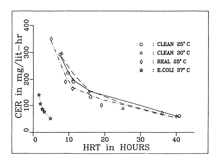
Figure 6. CER measurements vs HRT for four different systems
