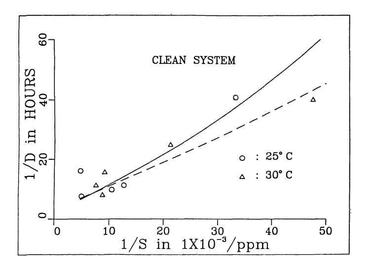
Figure 10. Comparison of experimental data and model predictions for 1/D VS 1/S for "clean system". Model predictions are represented by solid line for  $25^{\circ}$  C, and dashed for  $30^{\circ}$  C.
