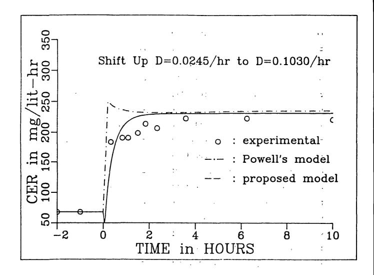
Figure 11. Comparison of CER data and model prediction of shift-up experiments.
