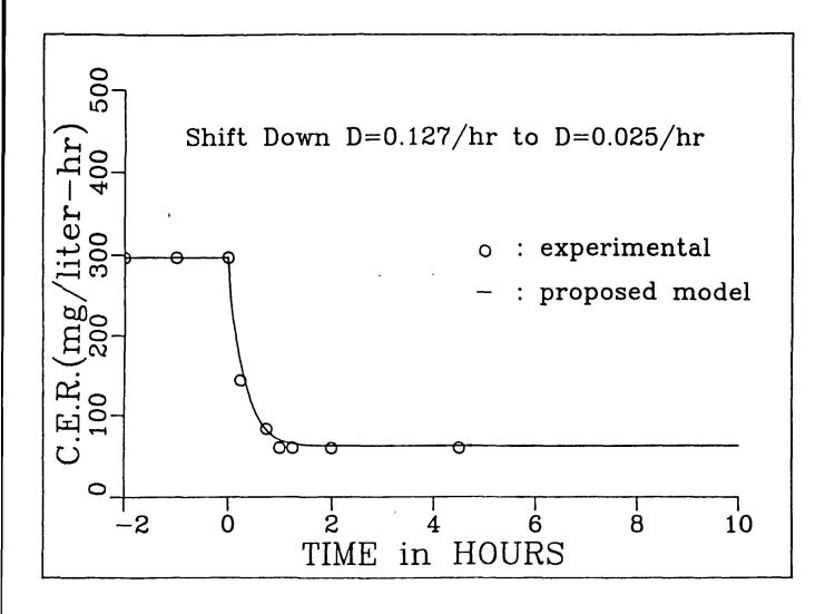
Figure 12. Comparison of CER data and model prediction of shift-down experiments.
