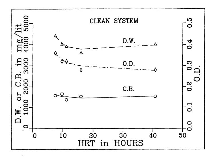
Figure 3. Comparison of different biomass estimation methods: Dry Weight(D.W.), Optical Density(O.D.), and Carbon Balance(C.B.)
