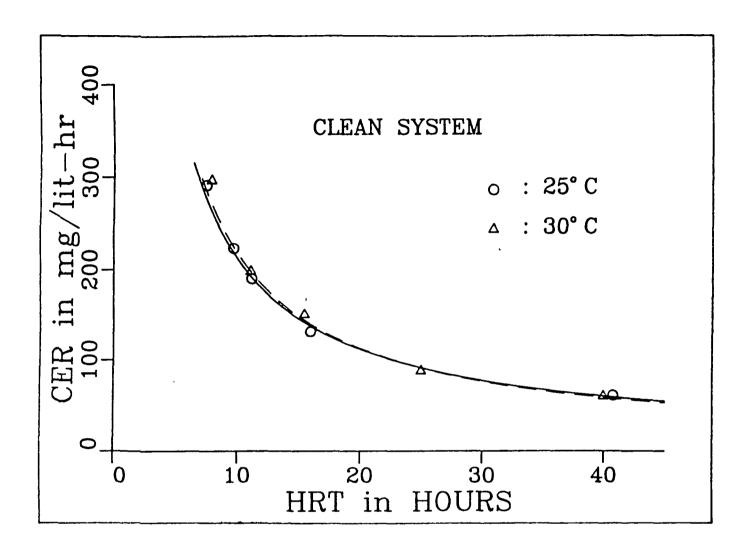
Figure 9. Comparison of experimental data and model predictions for CER for "clean system". Model predictions are represented by solid line for  $25^{\circ}$  C, and dashed line for  $30^{\circ}$  C.
