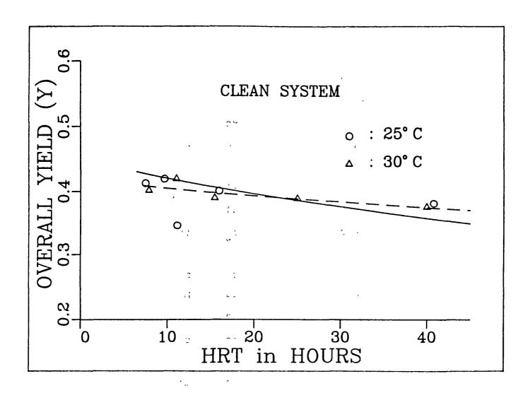
Figure 8. Comparison of experimental data and model prediction for overall yield(Y) for "clean system". Model predictions are represented by solid line for  $25^{\circ}$  C, and dashed line for  $30^{\circ}$  C.
