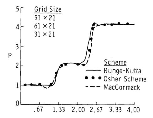
Figure 3. Plot of computed pressure at y = 0.25 for 2-D shock reflection.  $M_{\infty}$  = 2.9,  $\alpha$  = 29°.
