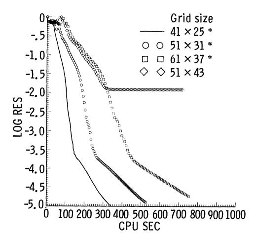
Figure 6. Convergence histories for different grid sizes for 2-D shock-reflection.  $M_{\infty}=2.9,~\alpha=23^{\circ}.$
