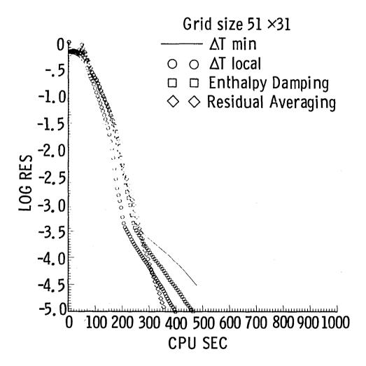
Figure 4. Convergence histories for different accelerating techniques for 2-D shock-reflection.  $M_{\infty}$  = 2.9,  $\alpha$  = 29°, Grid: 51 × 31.
