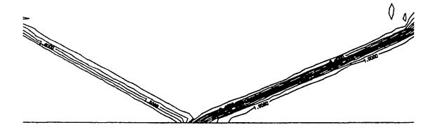
Figure 2. Contour plot of computed pressure for 2-D shock-reflection.  $M_{\infty} = \text{ 2.9, } \alpha = \text{ 29}^{\text{ 0}}.$
