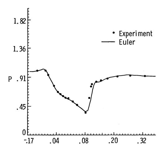
Figure 10. Comparison of computed and experimental surface pressure for 2-D nozzle.  $M_{in} \simeq 0.46$ .
