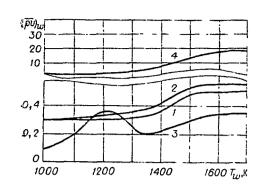
Relative effectiveness of the materials studied. 1,2--PG-50, ARV graphite, respectively; 3--tungsten; 4--chromium carbide  $(\overline{\rho v})_w = \frac{(\rho v)_w^*}{(\overline{\rho v})_w}$ , where  $(\rho v)_w^*$  --velocity of mass removal from the surface of the reference sample (B-1),  $(\rho v)_w$  --velocity of mass removal from the surface of the sample being studied.
