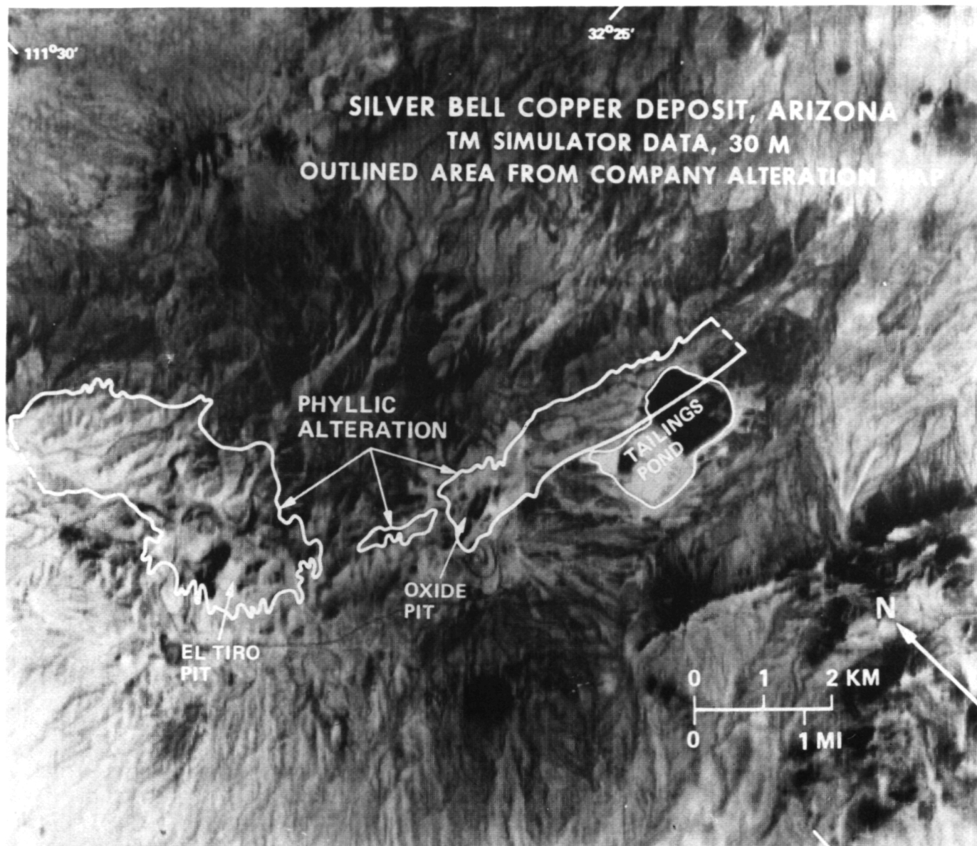
Figure 31. TMS data over the Silver Bell copper deposit, Arizona, resampled to 30-m pixels. Band ratios 1.65/2.2 \mu\text{m} , 0.66/0.56 \mu\text{m} , and 0.83/1.65 \mu\text{m} are displayed as red, green, and blue, respectively. The main alteration zone is displayed in yellow due to the presence of hydroxyl-bearing minerals and iron-oxide minerals. The phyllic alteration zone mapped from field and laboratory data is superimposed for comparison. (A color slide of this figure is inserted in the plastic holder at the end of this document.)
