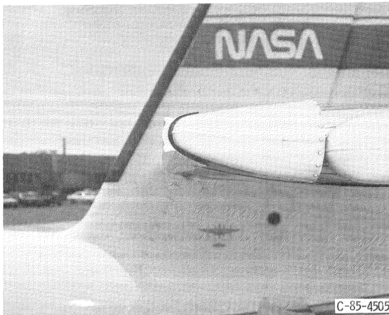
(b) Artificial "Light Glaze" ice shape.
