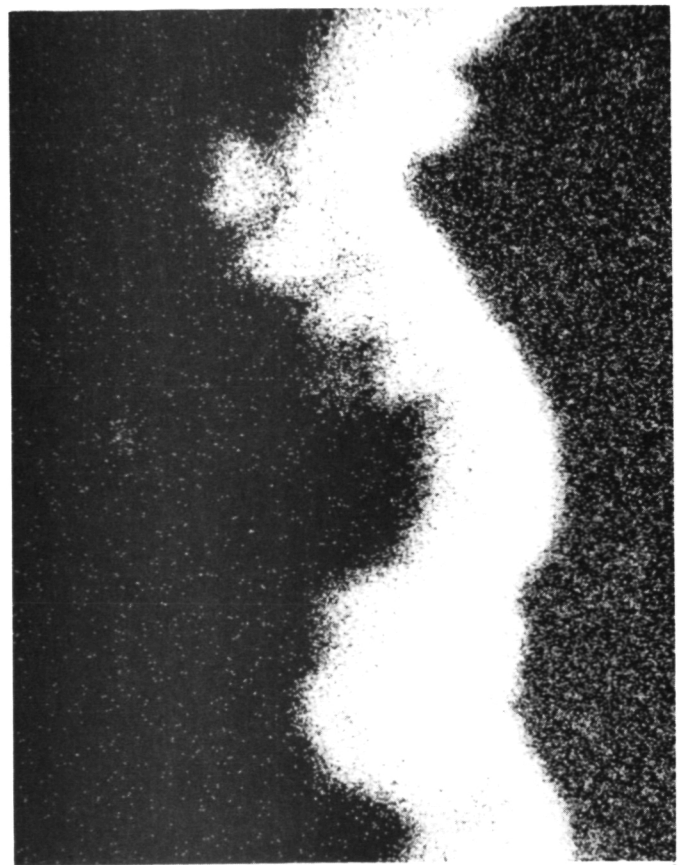
Figure 36 Cyclic Hot Corrosion Post-Test Specimen After 1000 hrs at 1650°F/ Long Cycle/35 ppm Artificial Sea Salt/1.3% SO 3
