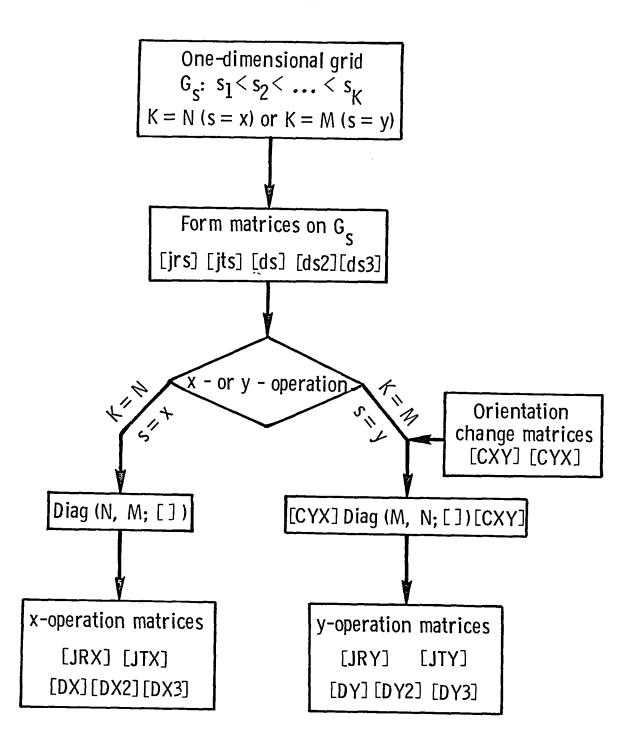
Figure 1. Flowchart illustrating the formation of matrices which approximate integrals and partial derivatives with respect to  $\mathbf{x}$  and  $\mathbf{y}$  on the rectangular grid  $\mathbf{G}$ .
