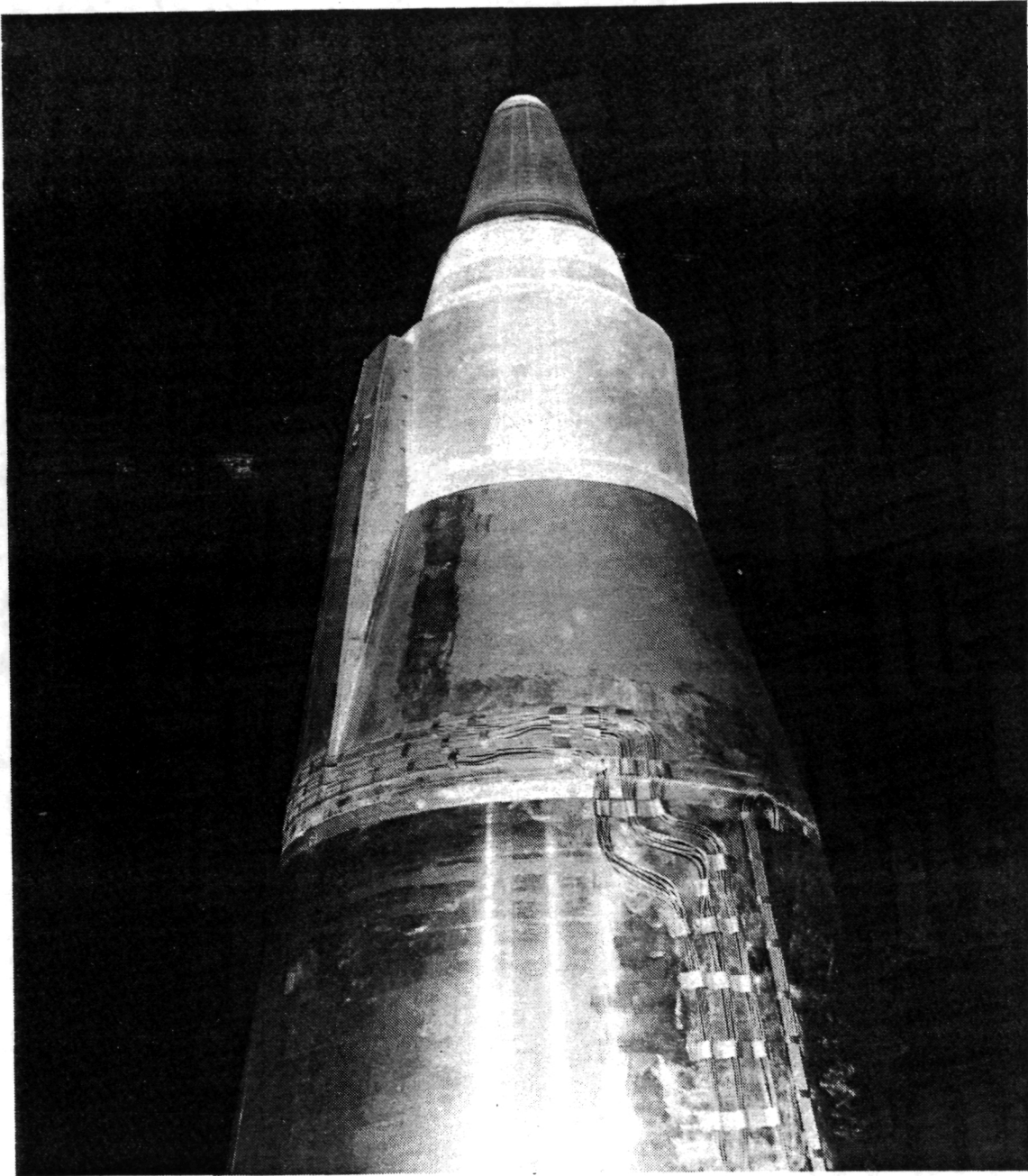
Figure 2.7. Photo of Unsuppressed Coannular Plug Nozzle With 180° Shield in Anechoic Test Facility, Configurations TAS-11 and TAS-12.
