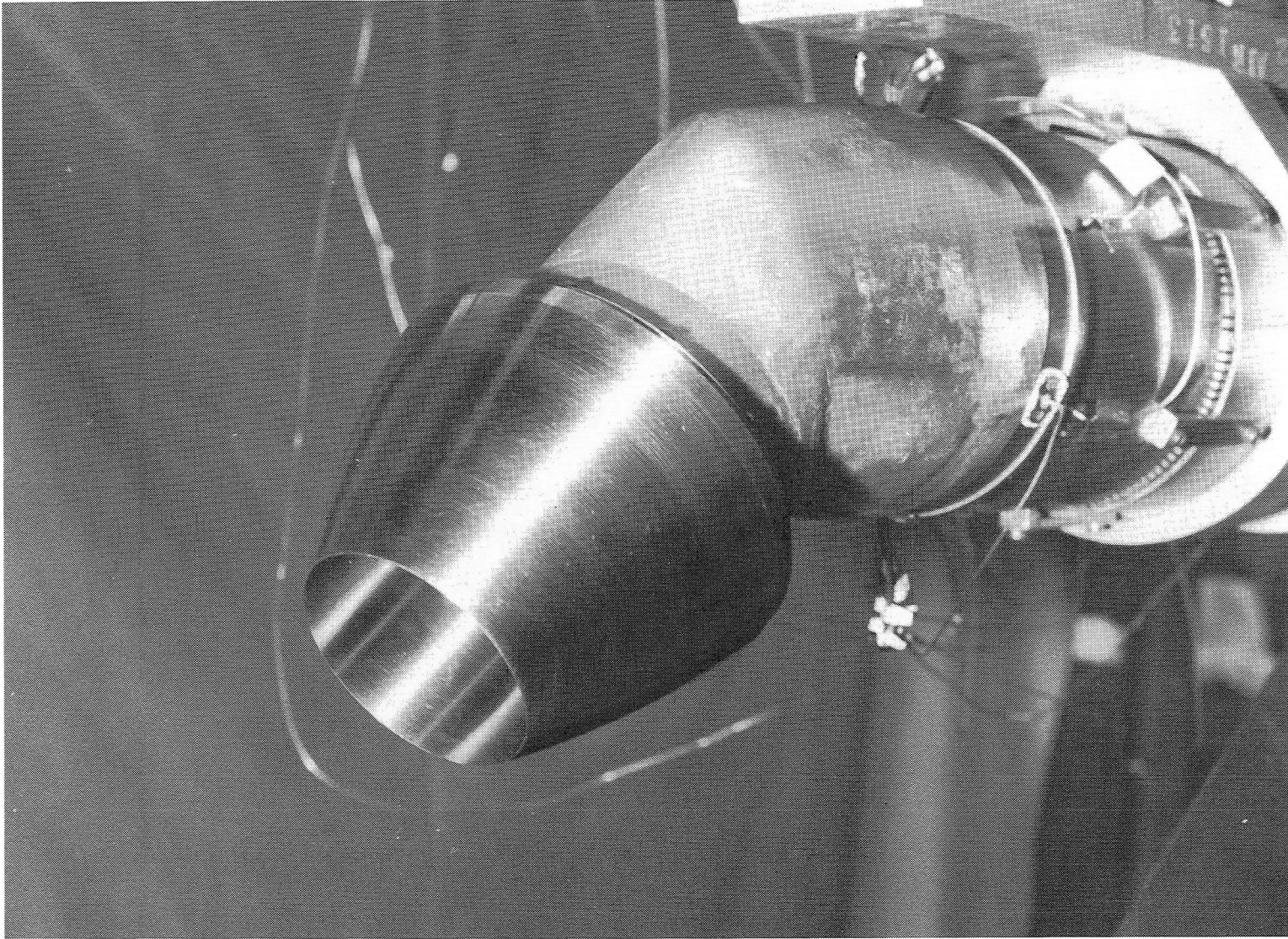
Figure 7.- Dry-power C-D nozzle configuration CDAD-D3 (with approach duct V-35) installed on single-engine propulsion simulation system.
