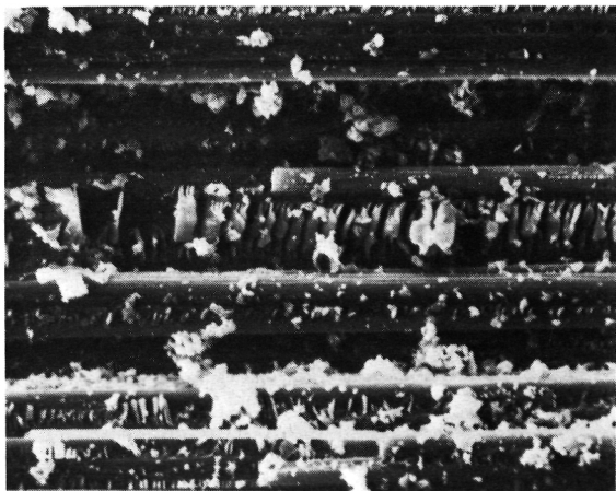
Figure 6. - Fracture characteristics associated with an overaged [\pm 15_2]_S laminate.
