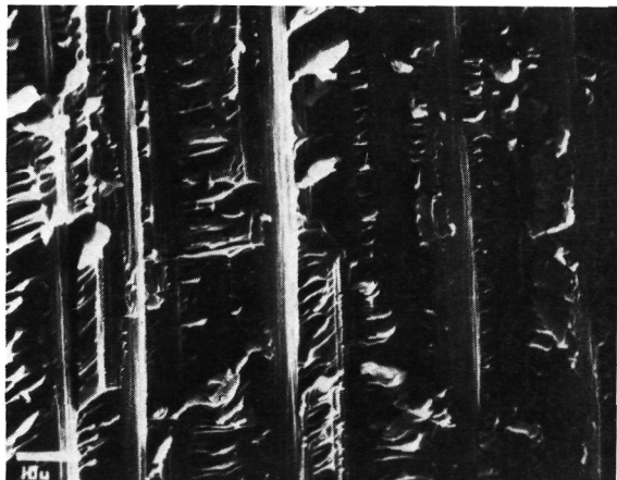
Figure 4. - The fractured specimens and typical microstructural characteristics for the [\_+45]_S laminate.
