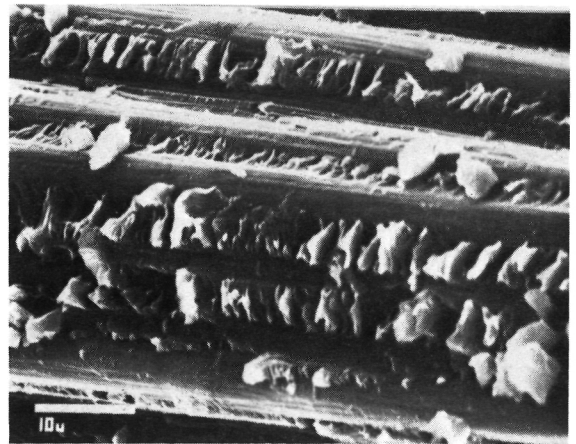
Figure 8. - Fracture characteristics associated with an overaged [\pm 45_2]_5 laminate.
