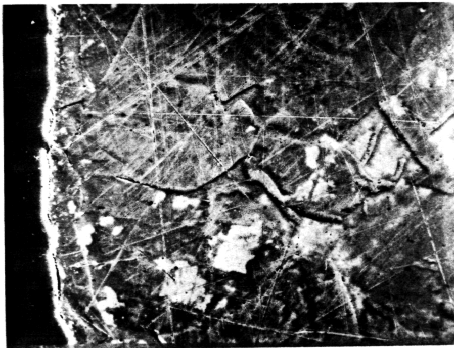
(b) IG initiation at surface - view B at 350X (SEM-34568)
