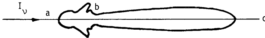
Figure 1-5. Sketch showing a typical scatter pattern. For most materials, the figure is rotationally symmetric about the slab.
